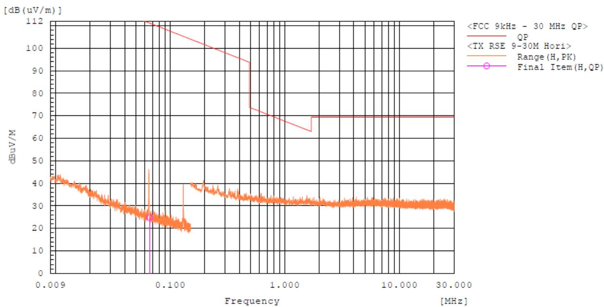
**Radiated Spurious Emission 9 kHz – 30 MHz (Antenna Position 180°) : ANTO (CH 11)**
