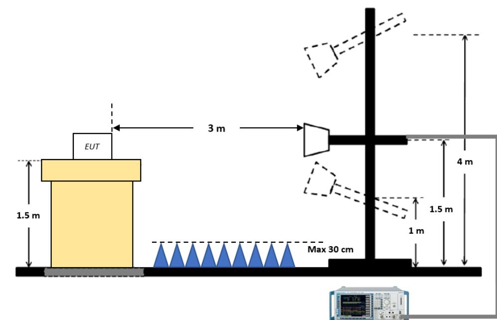
**TEST PROCEDURE OF RADIATED SPURIOUS EMISSION (BELOW 30 MHz)**
