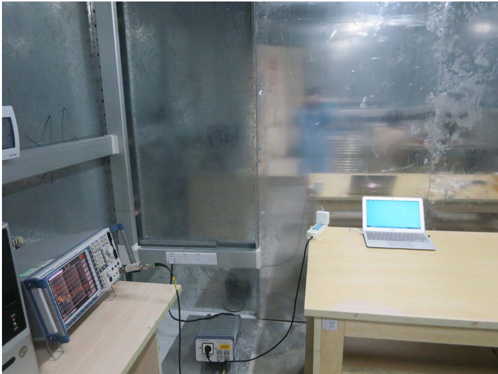
FCC RADIATED EMISSION TEST SETUP
