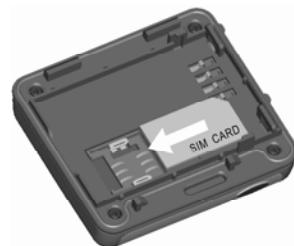
2. Disconnect and remove the battery. Insert the SIM card into the SIM holder in the direction as shown in picture.
