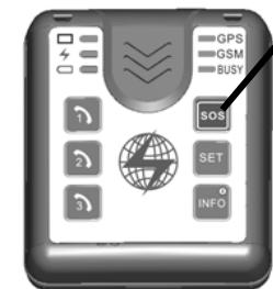
Press the SOS button for two seconds to trigger the emergency SMS.
