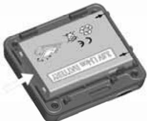
3. Place the battery in the compartment and reconnect it.
