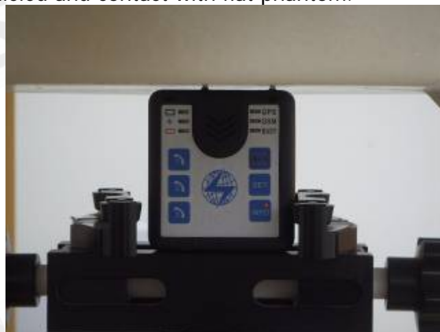
Fig.7 Top side of the EUT is paralleled and contact with flat phantom.
