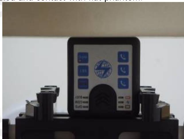
Fig.8 Bottom side of the EUT is paralleled and contact with flat phantom.
