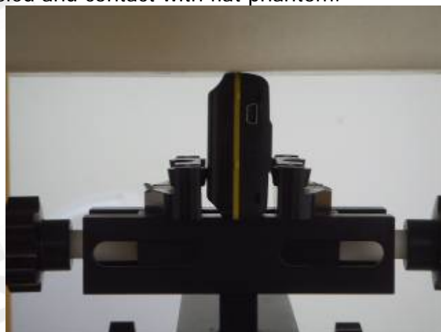
Fig.5 Right side of the EUT is Paralleled and contact with flat phantom.
