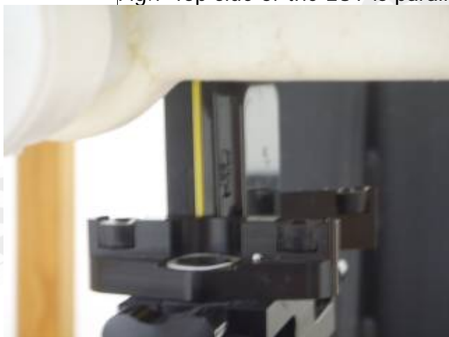
Fig.8 Bottom side of the EUT is paralleled and contact with flat phantom.
