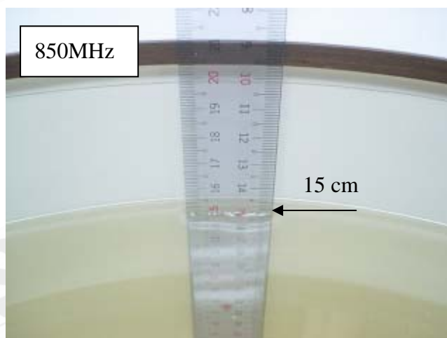
Fig.2.1 Photograph of the Tissue Simulant Fluid liquid depth 15cm for Flat (Body)
