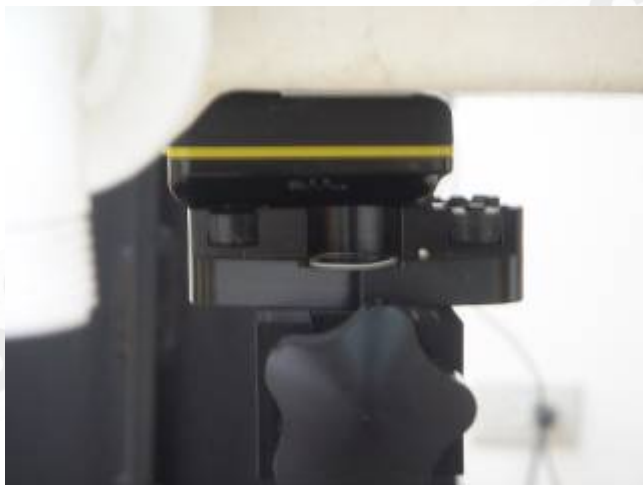
Fig.3 Front side of the EUT is paralleled and contact with flat phantom.
