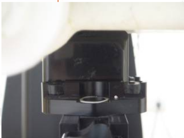
Fig.6 Left side of the EUT is paralleled and contact with flat phantom.
