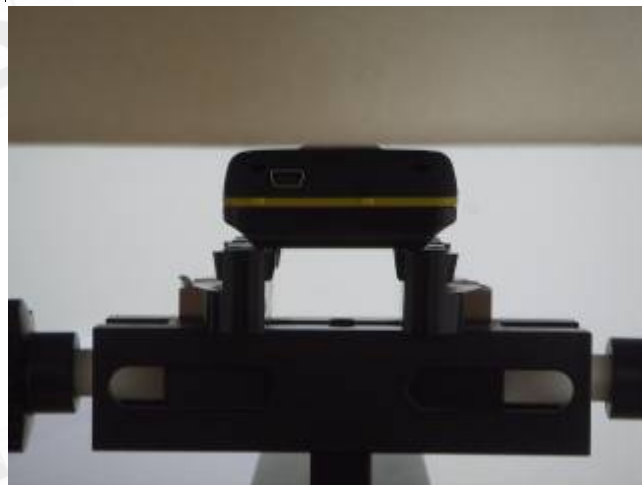
Fig.3 Front side of the EUT is paralleled and contact with flat phantom.
