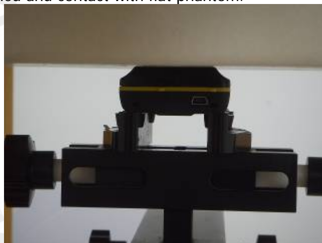
Fig.4 Back side of the EUT is paralleled and contact with flat phantom.
