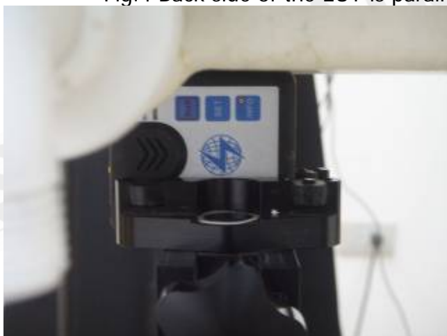
Fig.5 Right side of the EUT is Paralleled and contact with flat phantom.
