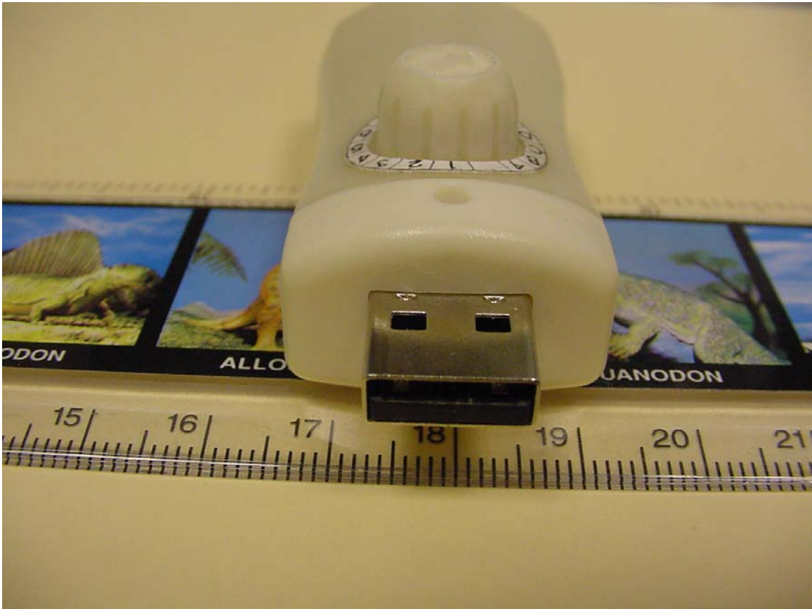
End of EUT showing USB connector (used for power only)
