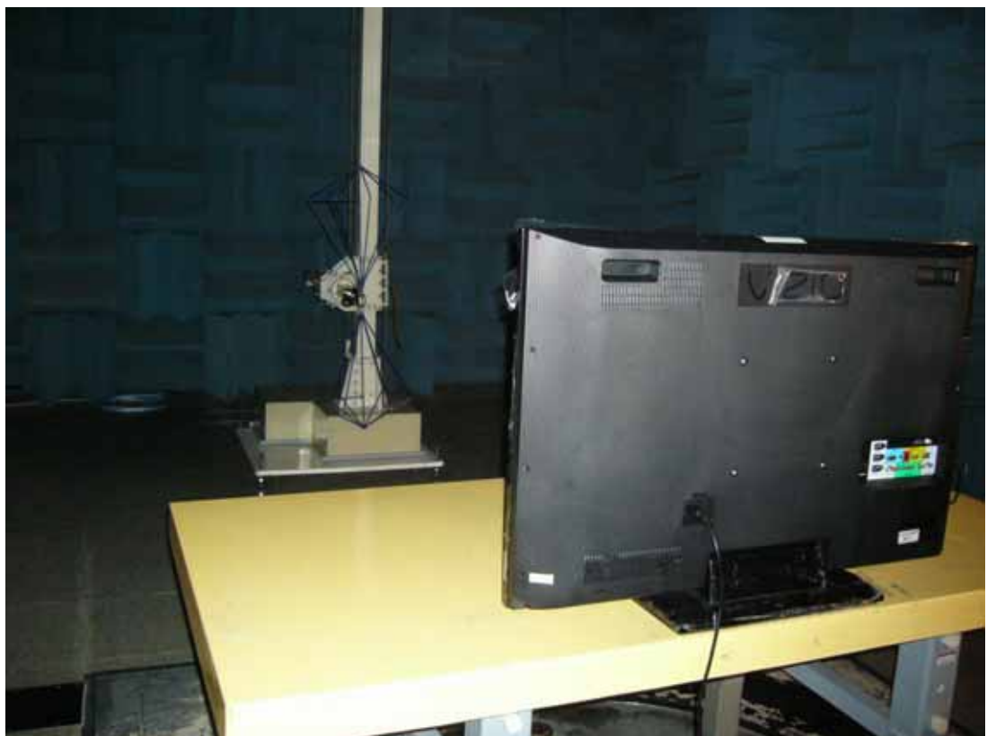
BACK VIEW OF RADIATED MEASUREMENT
