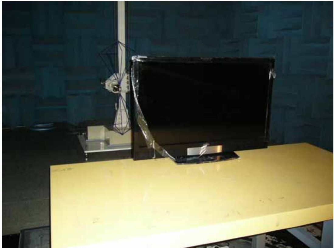
FRONT VIEW OF RADIATED MEASUREMENT
