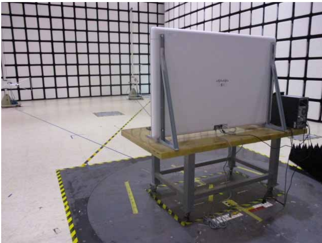
Back View of Radiated Measurement
