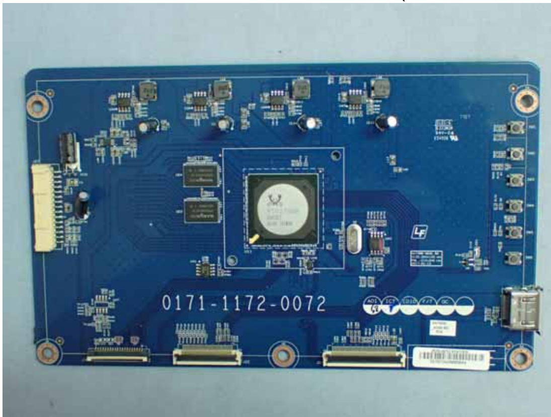
Figure 17 Internal View (Control Board, Front View)
