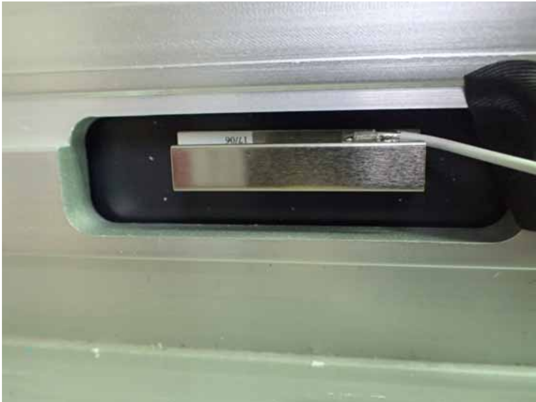
Figure 7 Internal View (Antenna View)
