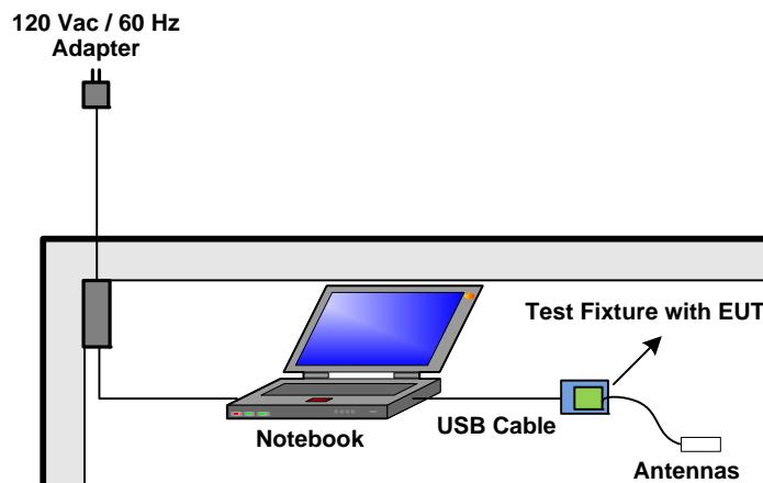
**Test Setup Diagram - Radiated Test (Above 1GHz)**
