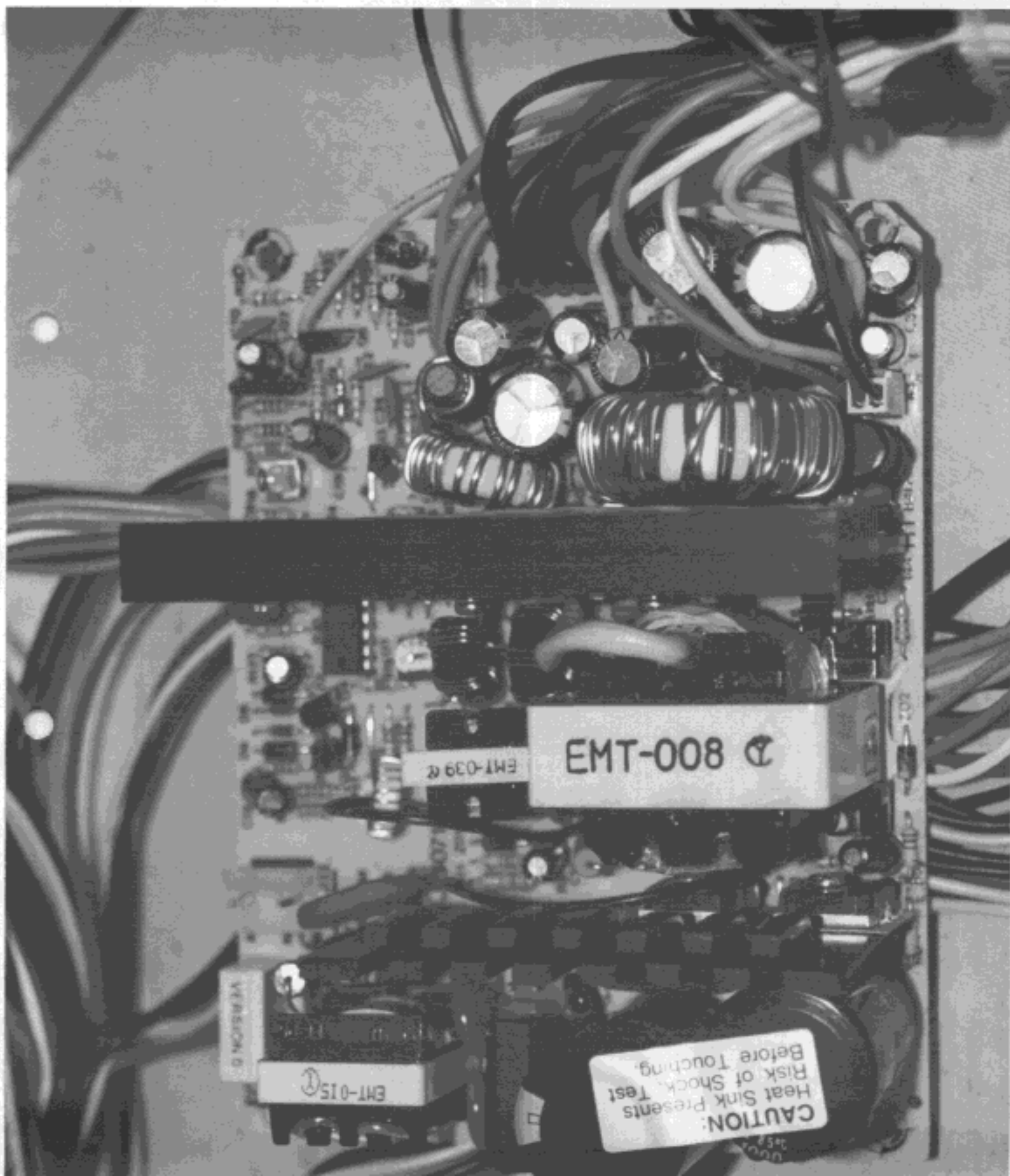
Figure 19 Switching Power Supply (PCB View, Component Side)
