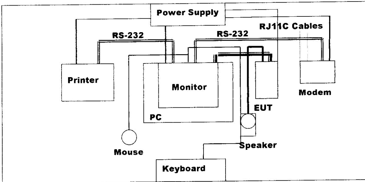
During testing the EUT(External CD-RW)r) was connected to Compaq PC's SCSI I/O port. So there is need for additional SISC Card. A speaker was connected to audio jack of EUT. A modem was connected to the series port and a printer was connected to the parallel port. Two telephone line(RJ11C cables) connected to the Phone Jack of modem and the Line Jack of modem. A keyboard and mouse were connected to the PS/2 port.
