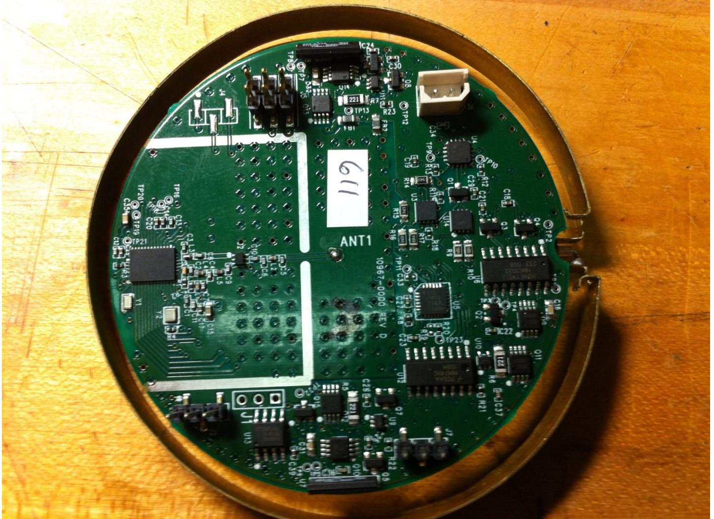
Figure 5 Circuit Card Assembly with Loop Antenna Visible
