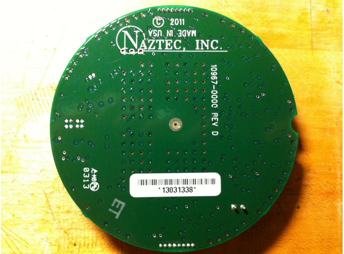
Figure 8 Circuit Card Assembly without Loop Antenna - Non-component Side
