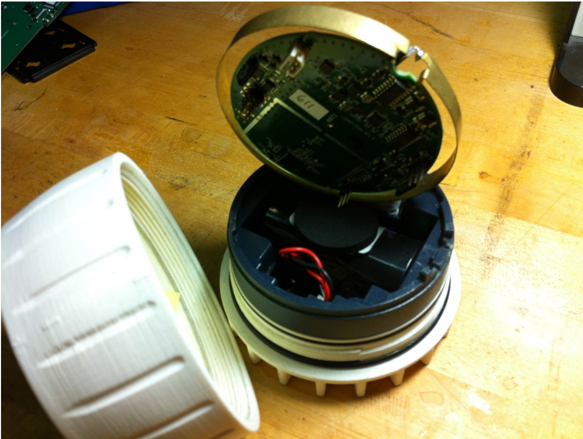
Figure 3 Circuit Board Assembly Lifted to Reveal Component Side and Battery Compartment
