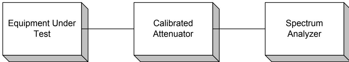
**Para. No. 2.993 - Field Strength of Spurious Radiation**
