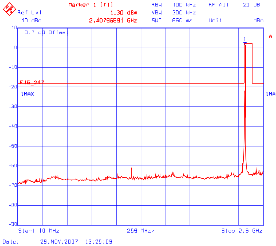
Plot 6.8.5.2.1(i) Spurious RF Conducted Emissions Transmitter Frequency: 2405 MHz
