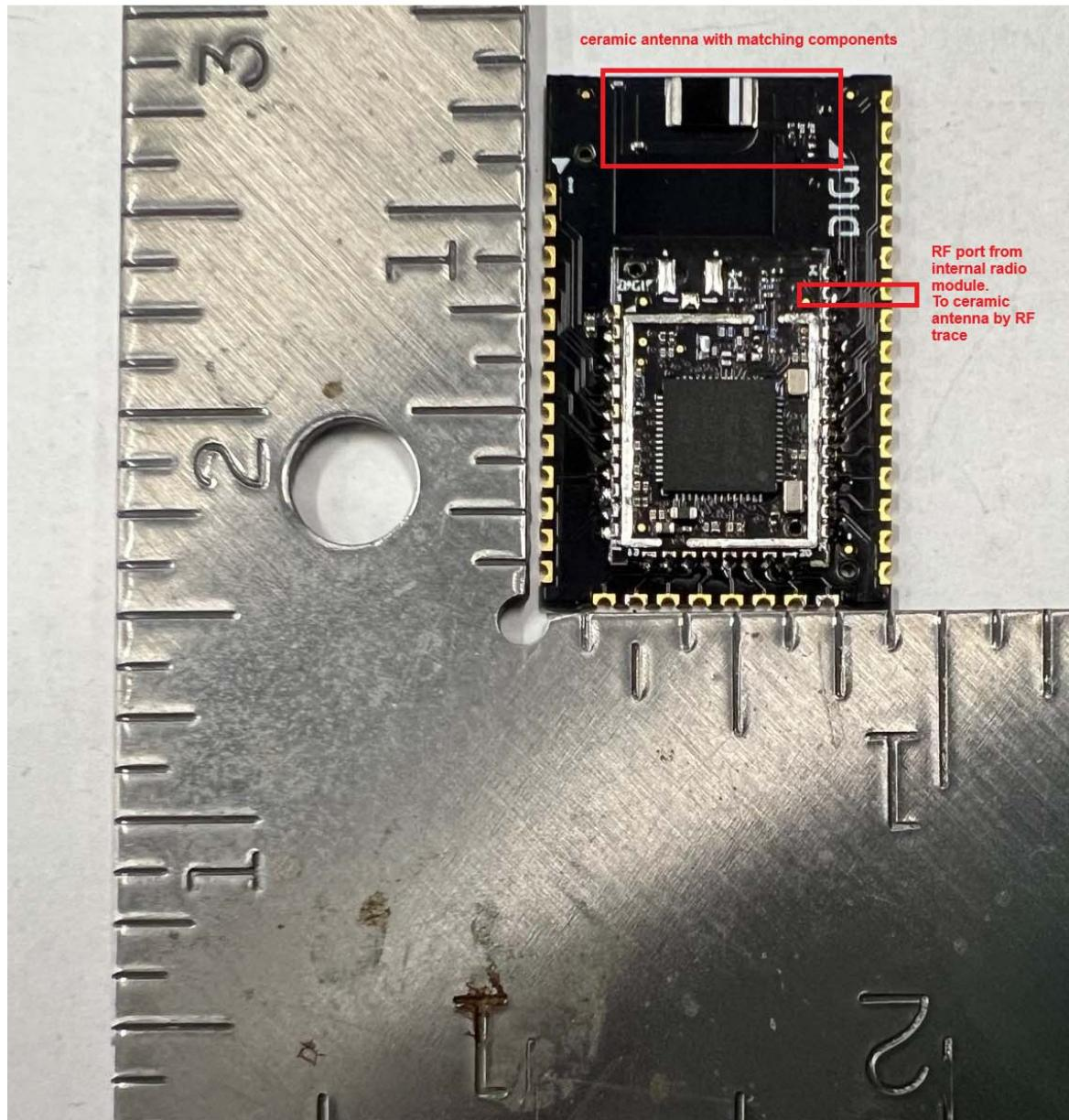
ceramic antenna with matching components
