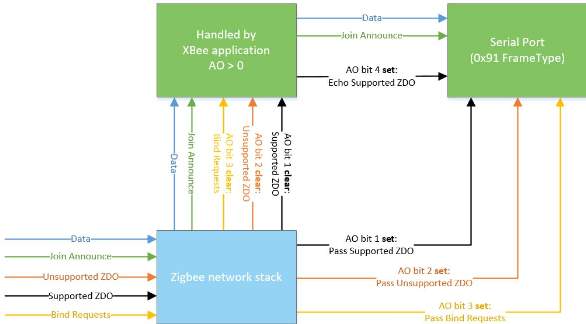
When a ZDO message is received on endpoint 0 and profile ID 0, the cluster ID indicates the type of ZDO message received. The first byte of payload is generally a sequence number that corresponds to a sequence number of a request. The remaining bytes are set as defined by the ZDO. Similar to a ZDO request, all multi-byte values in the response are in little endian byte order.
