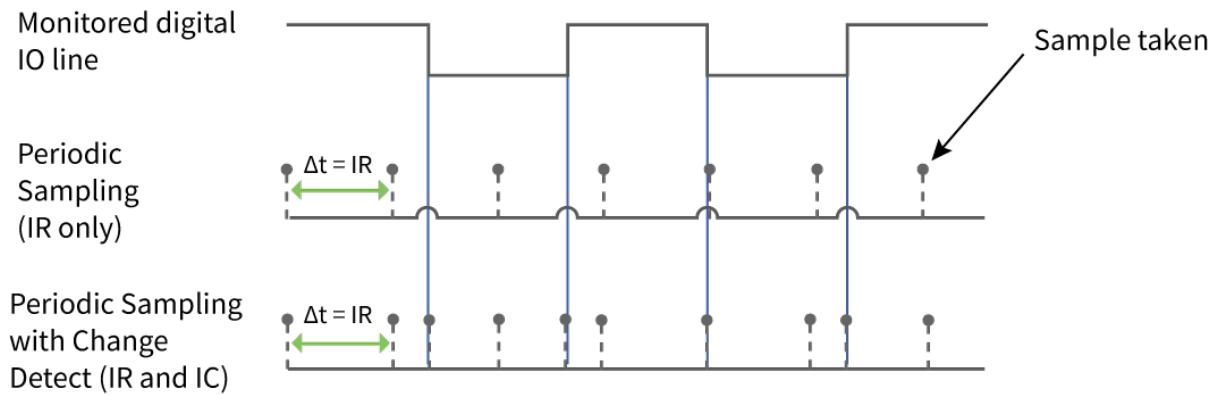
**Note** Use caution when combining change detect sampling with **sleep modes**. **IC** only causes a sample to be generated if a state change occurs during a wake period. If the device is sleeping when the digital transition occurs, then no change is detected and an I/O sample is not generated. Use periodic sampling with **IR** in conjunction with **IC** in this instance, since **IR** generates an I/O sample upon wakeup and ensures that the change is properly observed.
