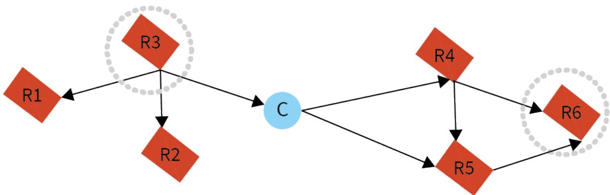
When the destination node receives a route request, it compares the 'path cost' field against previously received route request commands. If the path cost stored in the route request is better than any previously received, the destination node transmits a route reply packet to the node that originated the route request. Intermediate nodes receive and forward the route reply packet to the source node (the node that originated route request).
