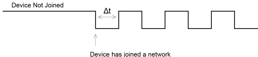
The associate pin can indicate the joined status of a device. Once the device has joined a network, the associate pin toggles state at a regular interval ( $\Delta t$ ). Use the **LT** command to set the time.
