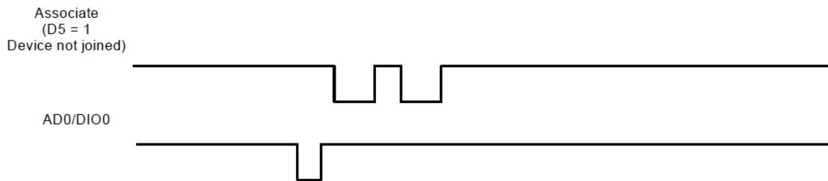
The following image illustrates the behavior pressing the button once on a remote device, causing a broadcast node identification transmission to be sent. All devices that receive this transmission blink their associate pin rapidly for one second if the associate LED functionality is enabled (**D5 = 1**).
