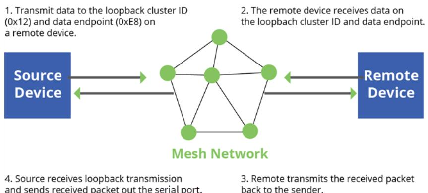
The configuration steps for sending data to the loopback cluster ID depend on what mode the device is in. For details on setting the mode, see [AP \(API Enable\)](#). The following sections list the steps based on the device's mode.
