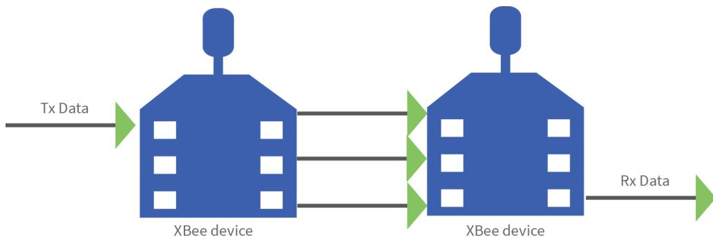
The transmit frame can include up to 255 bytes of data broken up into multiple transmissions and reassembled on the receiving side. If one or more of the fragmented messages are not received by the receiving device, it drops the entire message, and the sender indicates a transmission failure in [Extended Transmit Status - 0x8B](#).
