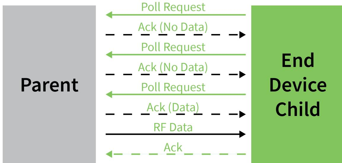
If the end device receives the acknowledgment and finds that the parent has no data for it, the end device can return to idle mode or sleep. Otherwise, it remains awake to receive the data. This polling mechanism allows the end device to enter idle mode and turn its receiver off when RF data is not expected in order to reduce current consumption and conserve battery life.
