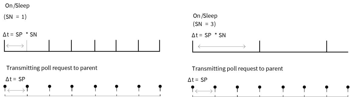
Setting **SN** > 1 allows the device to silently poll for data without asserting On/Sleep. If RF data is received when polling, On/Sleep will immediately assert.
