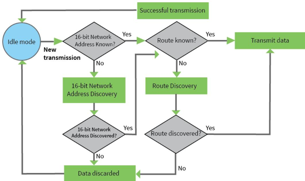
When Zigbee data is transmitted from one node to another, the destination node transmits a network-level acknowledgment back across the established route to the source node. This acknowledgment packet indicates to the source node that the destination node received the data packet. If the source node does not receive a network acknowledgment, it retransmits the data.
