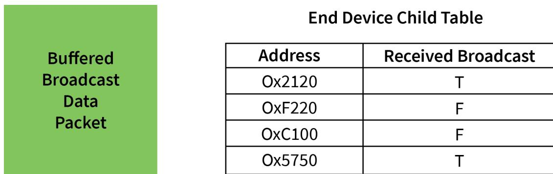
When an end device sends data to its parent that is destined for a remote device in the network, the parent buffers the data packet until it can establish a route to the destination. The parent may perform a route or 16-bit address discovery of its end device children. Once a route is established, the parent sends the data transmission to the remote device.
