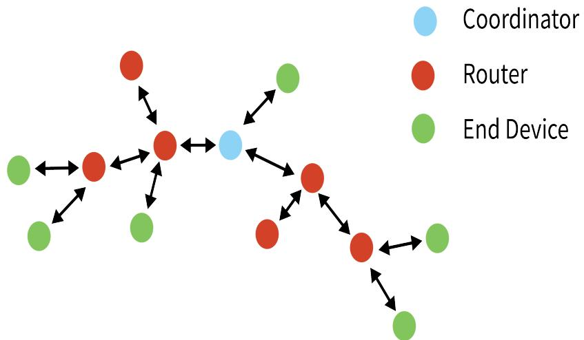
**Note** Each Zigbee network must be formed by one, and only one, coordinator and at least one other device (router or end device).
