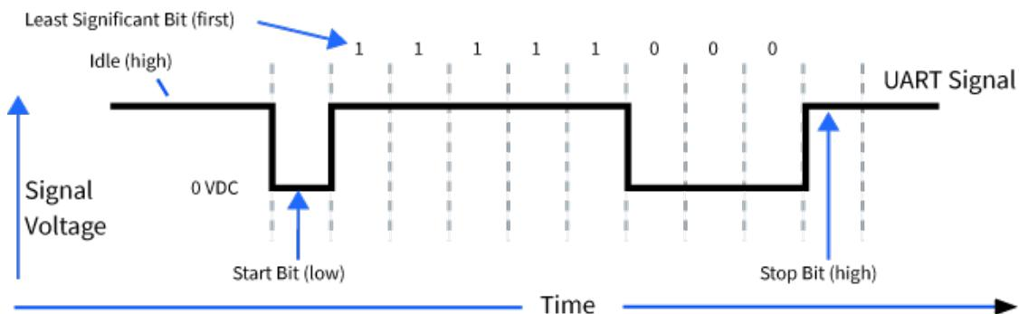
You can configure the UART baud rate, parity, and stop bits settings on the device with the **BD**, **NB**, and **SB** commands respectively. For more information, see [UART interface commands](#).
