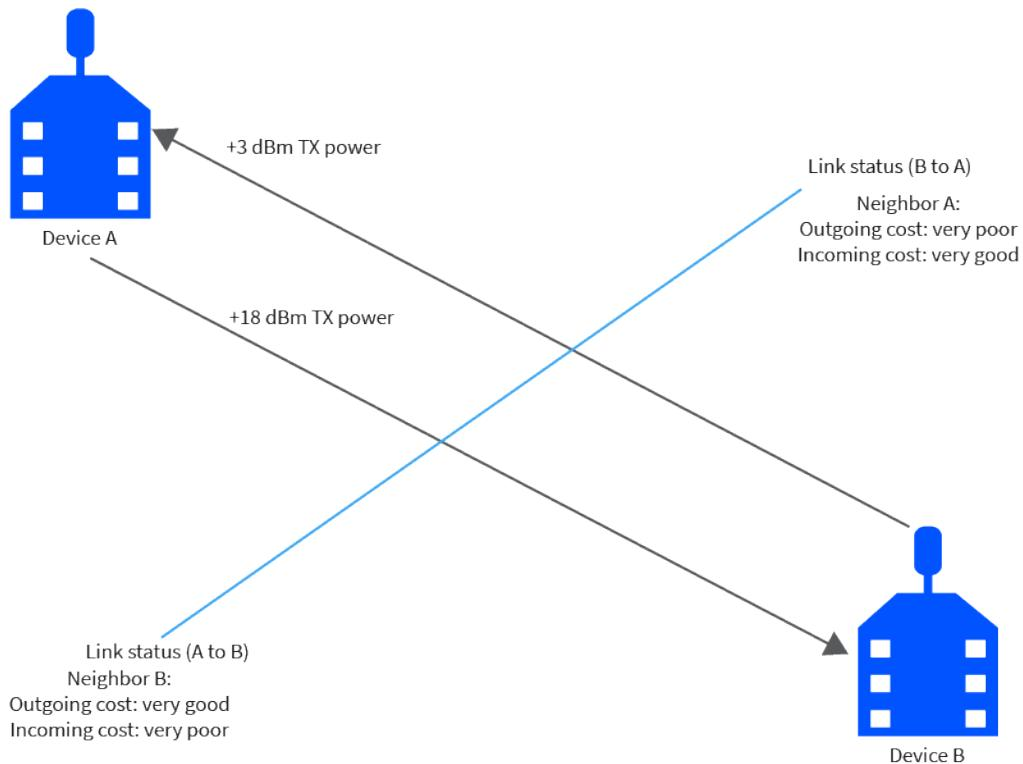
This mechanism enables devices A and B to recognize that the link is not reliable in both directions and select a different neighbor when establishing routes. Such links are called asymmetric links, meaning the link quality is not similar in both directions.
