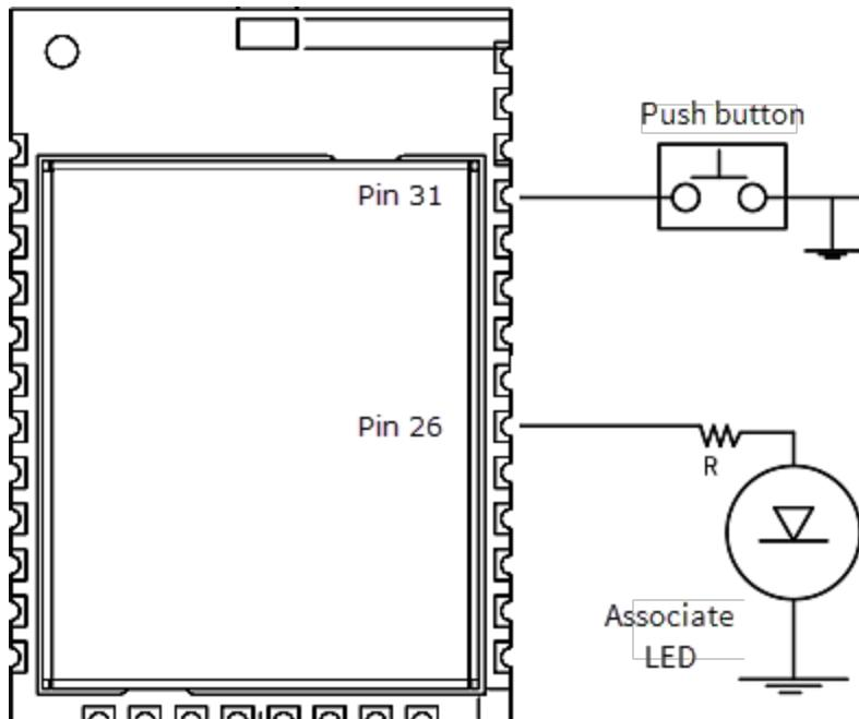
A pushbutton and an LED can be connected to the Micro device to support the commissioning pushbutton and associate LED functionalities.
