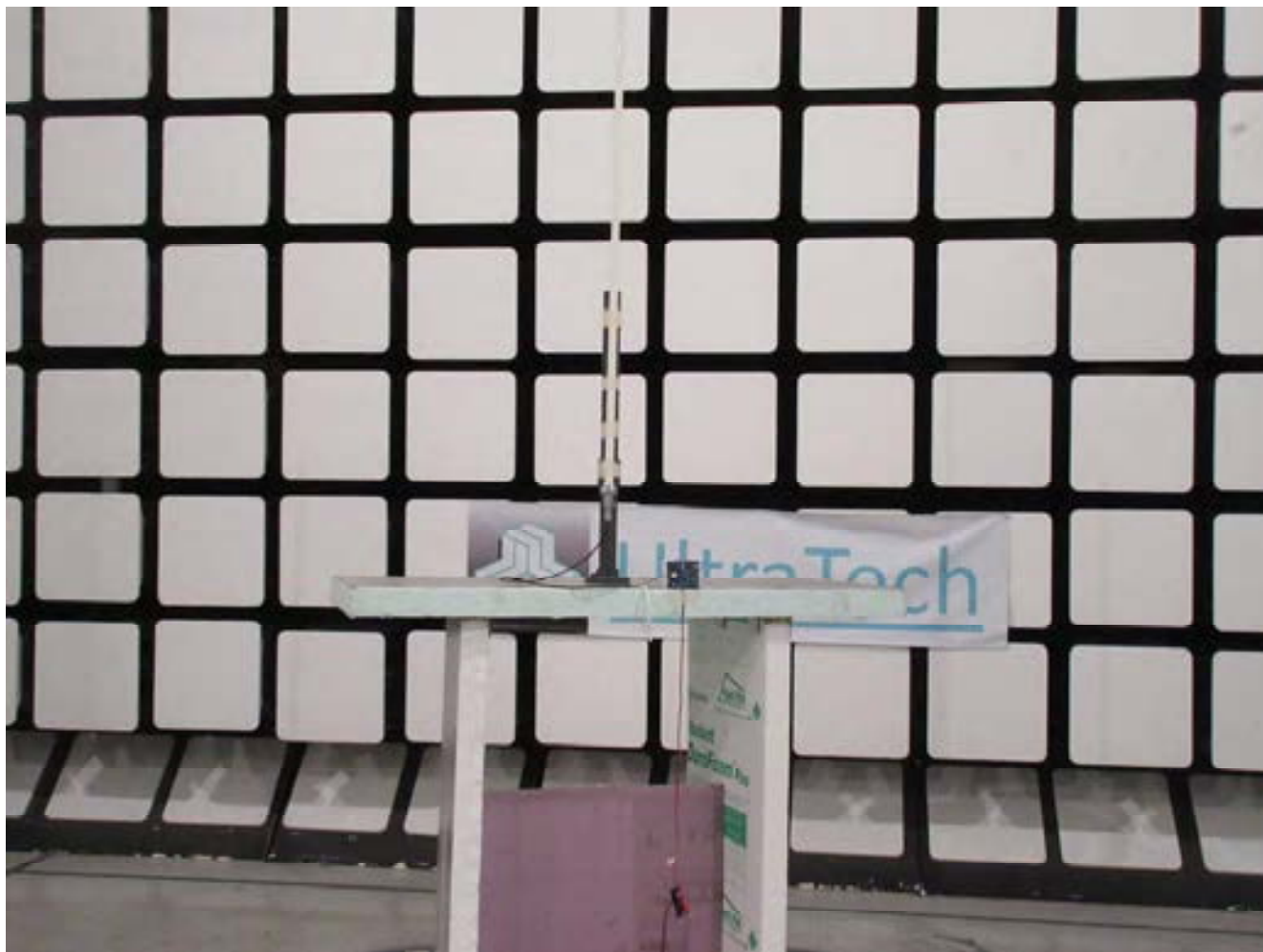
Radiated Emissions @ 3 m EUT with 15 dBi Omni Directional Antenna, Orthogonal Position 2
