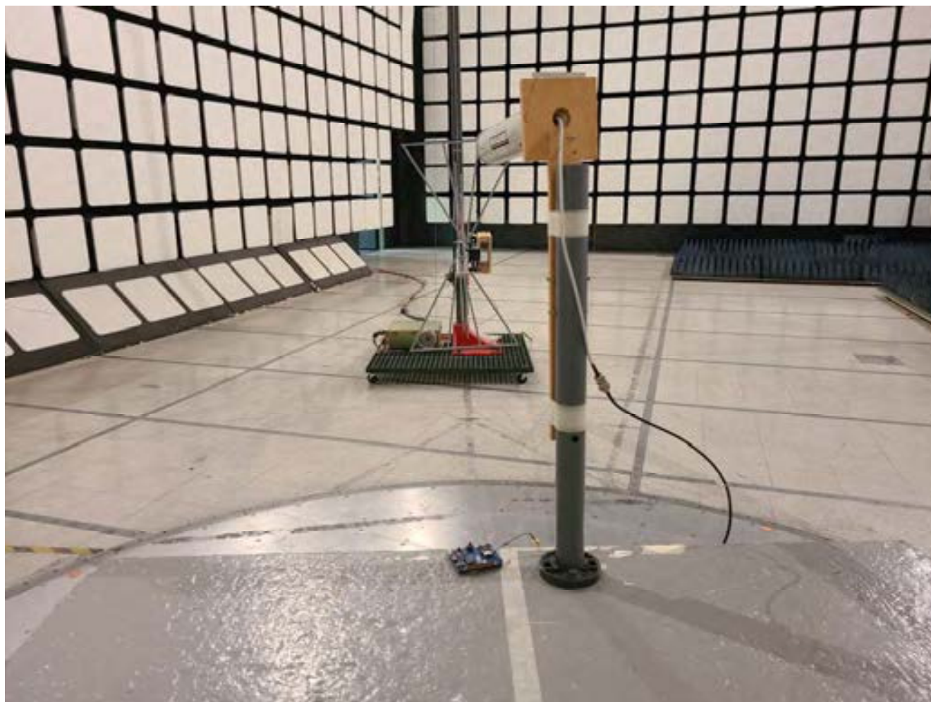
Radiated Emissions @ 3 m EUT with 15 dBi Yagi Antenna, Orthogonal Position 1
