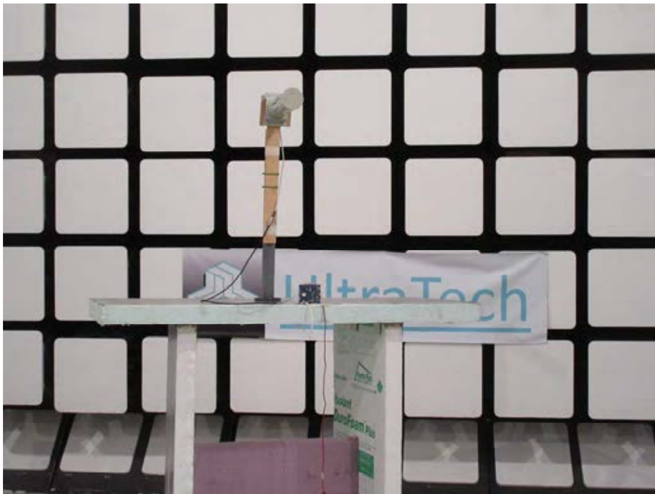
Radiated Emissions @ 3 m EUT with 15 dBi Yagi Antenna, Orthogonal Position 2
