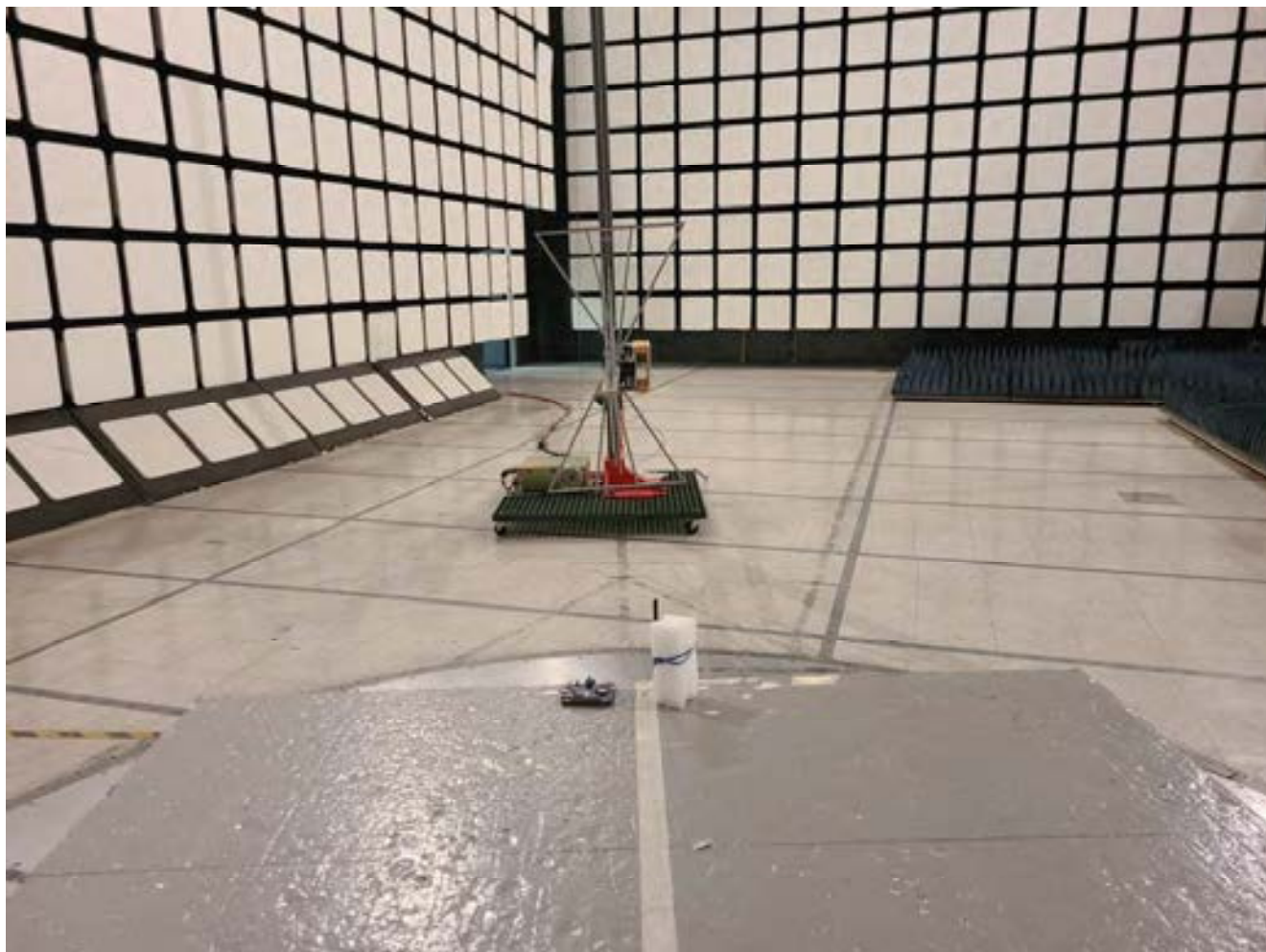
Radiated Emissions @ 3 m EUT with 2.1 dBi Dipole Antenna, Orthogonal Position 1
