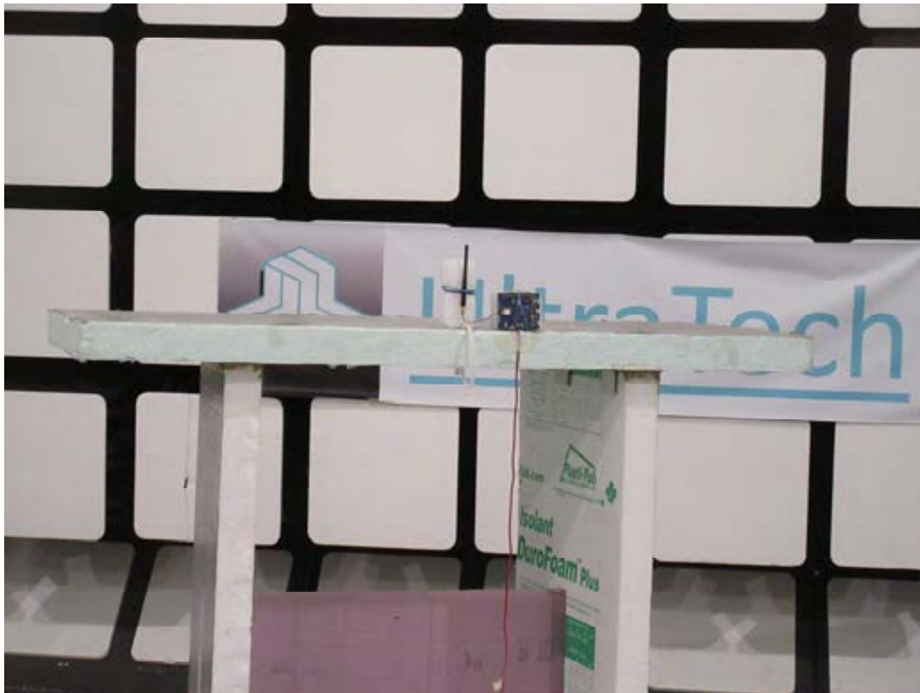
Radiated Emissions @ 3 m EUT with 2.1 dBi Dipole Antenna, Orthogonal Position 2
