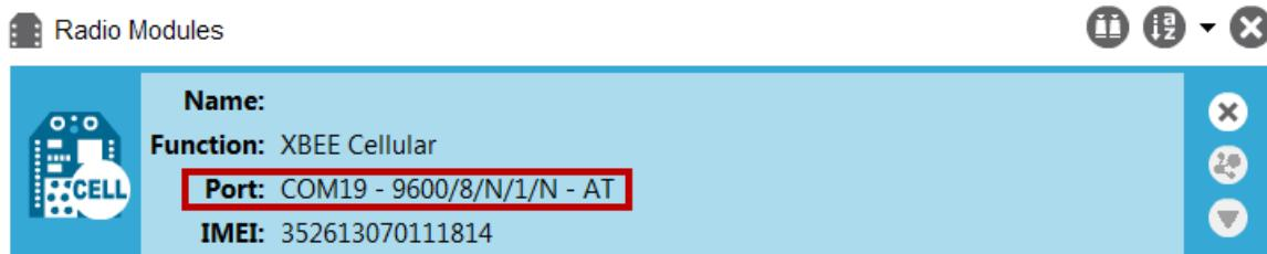
7. Type the baud rate and press **Enter**. You must match the device's current baud rate. XCTU provides the current baud rate in the **BD Baud Rate** field. In this example you would type **9600**.
