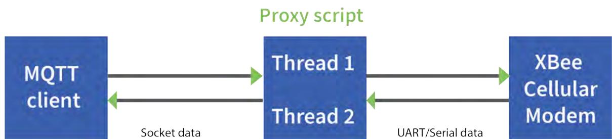
The thread that reads the serial port forwards any data received onward to the client socket, and the thread reading the client socket forwards any data received onward to the serial port. This is represented in the figure above.
