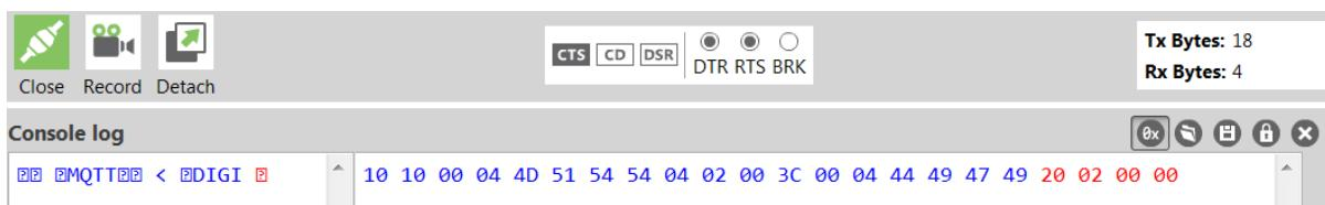
You can verify the response from the broker as a CONNACK by comparing it to the structure of a CONNACK packet in the MQTT documentation, which is available at [http://docs.oasis-open.org/mqtt/mqtt/v3.1.1/os/mqtt-v3.1.1-os.html#\\_Toc398718081](http://docs.oasis-open.org/mqtt/mqtt/v3.1.1/os/mqtt-v3.1.1-os.html#_Toc398718081).
