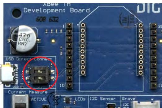
4. Configure the device for USB Direct access.
