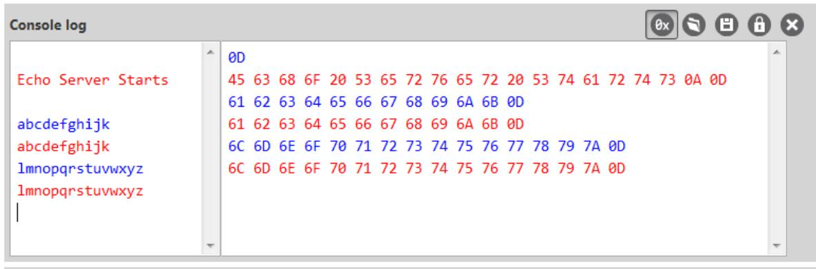
The screenshot shows the 'Console log' window in the XCTU software. The left pane displays text input, and the right pane shows the corresponding serial output. The output consists of several lines of hex and ASCII data, primarily in red, representing the echo server's response to the input. The input lines are in black.
