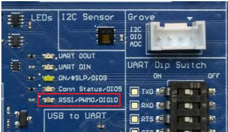
1. Note the **DIO10** LED on the XBee board. The following image highlights it in a red box. The LED is normally off.
