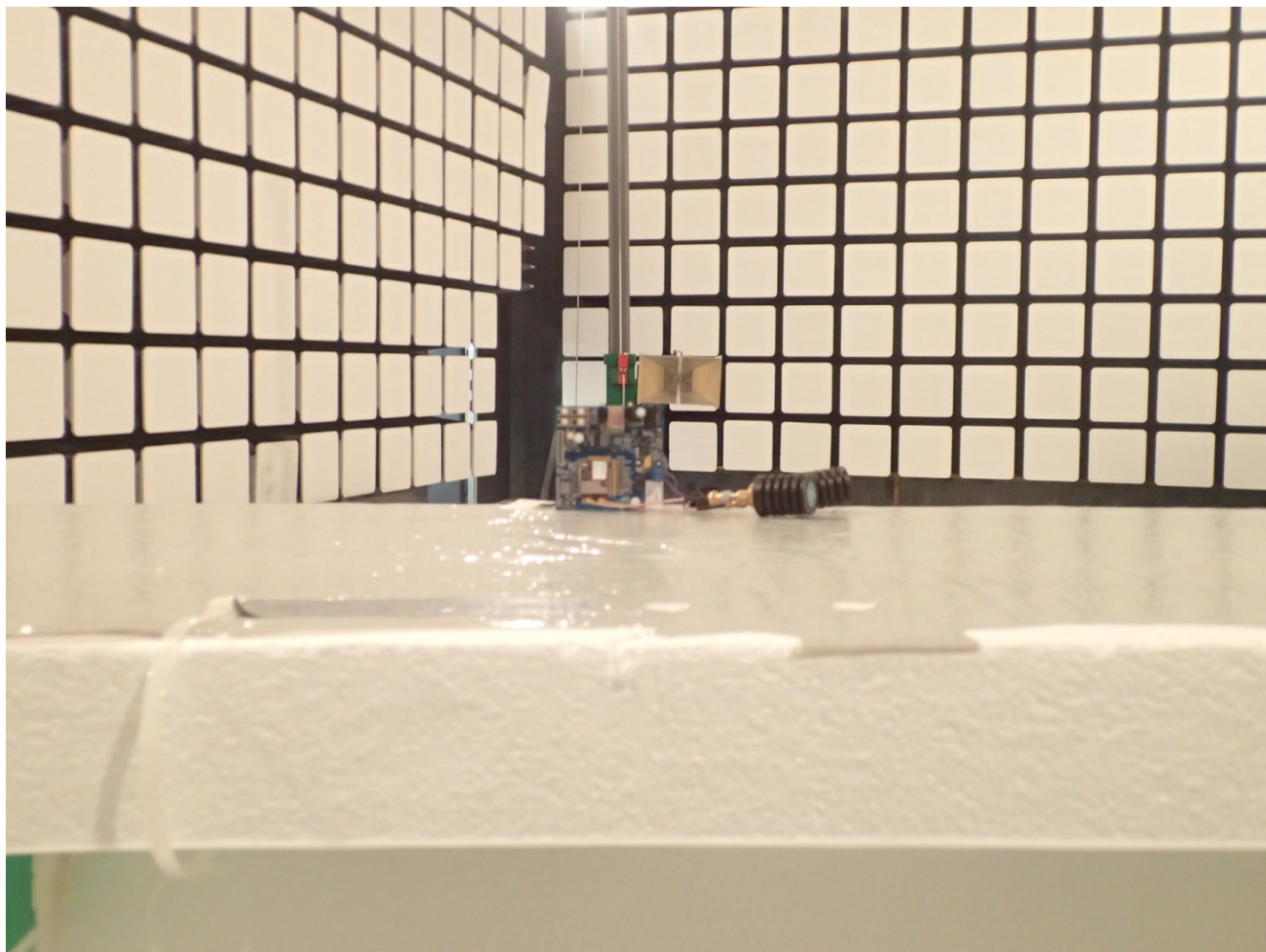
Radiated Emissions @ 3 m, Orthogonal Position 3
