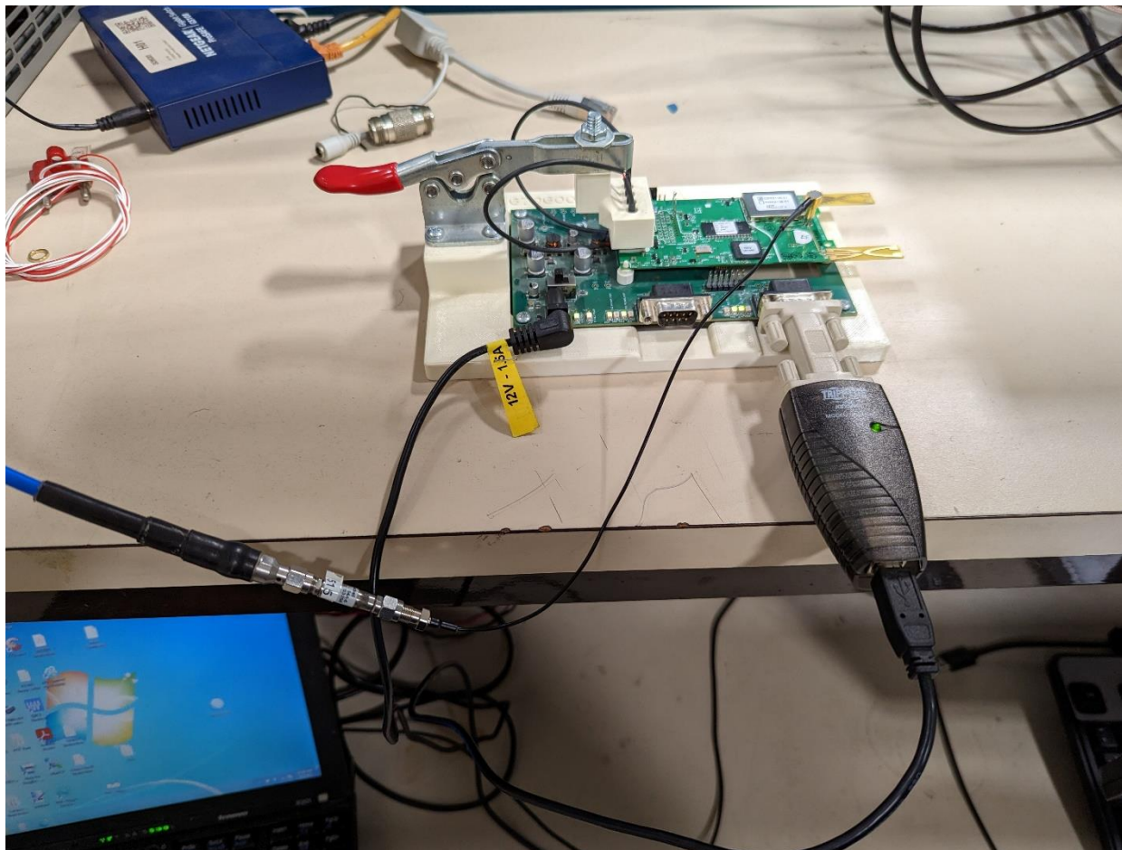
DIGI107 RF Conducted Setup
