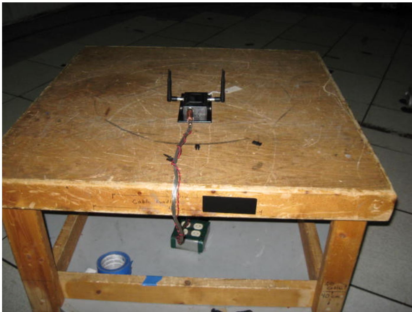
Test-setup photo(s): Radiated measurements, 2 dBi antenna
