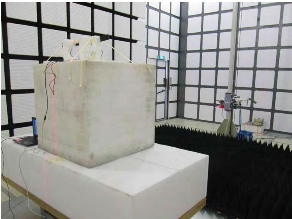
**ANTENNA PORT CONDUCTED RF MEASUREMENT SETUP**
