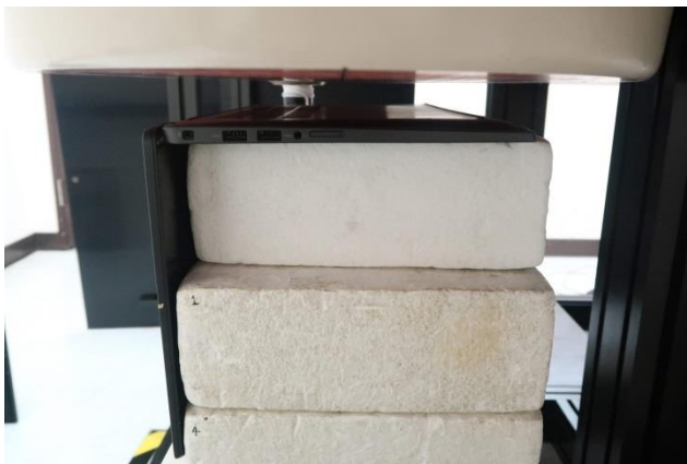
Bottom of Laptop, Test Separation 24 mm
