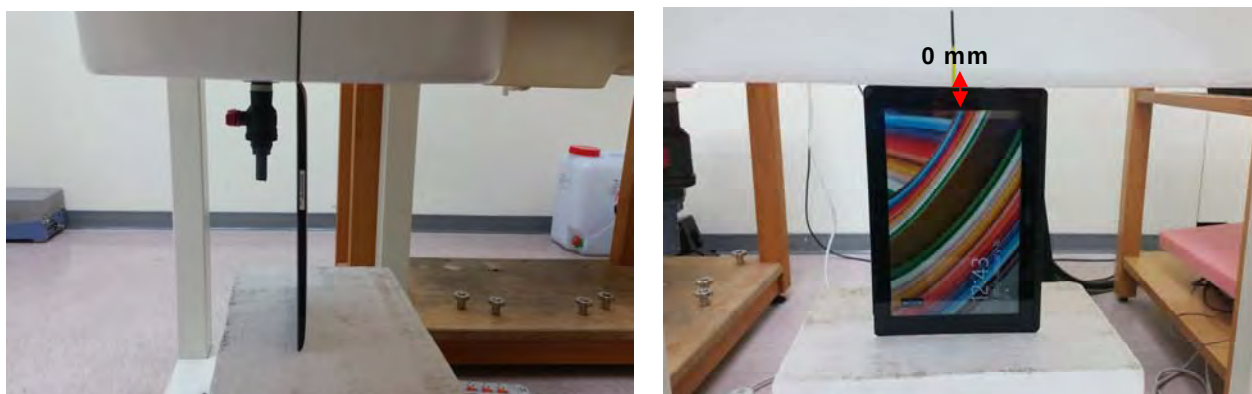
Fig.5 EUT Right side to flat phantom
