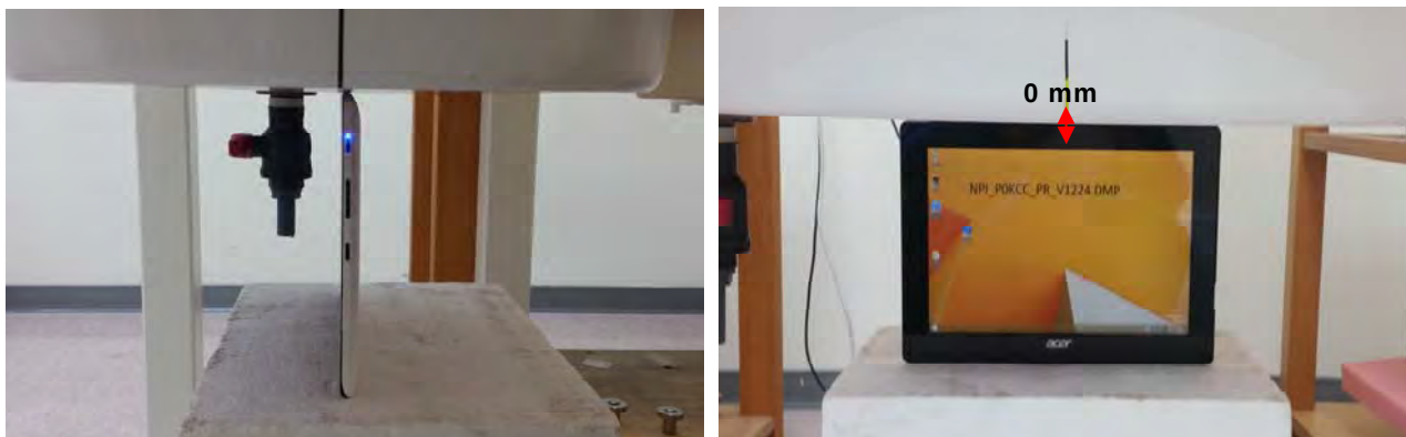
Fig.4 EUT Top side to flat phantom
