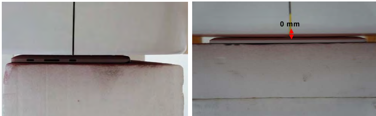
Fig.3 EUT Lap-held mode to flat phantom
