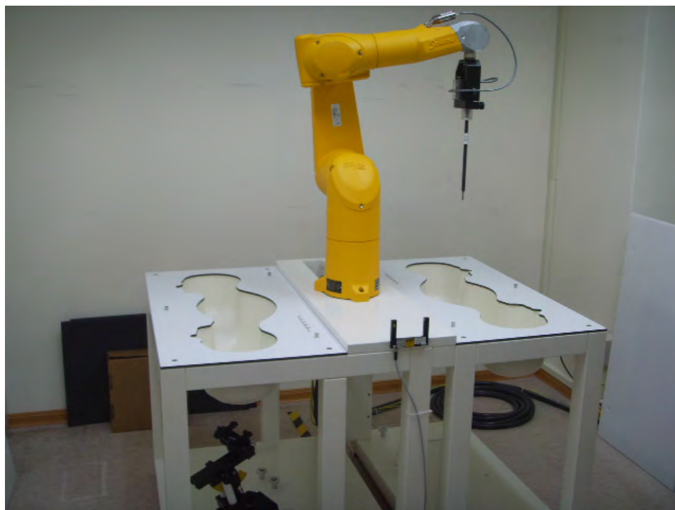
Fig.1 Photograph of the SAR measurement system
