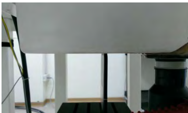
Fig.3 EUT Back side mode to flat phantom
