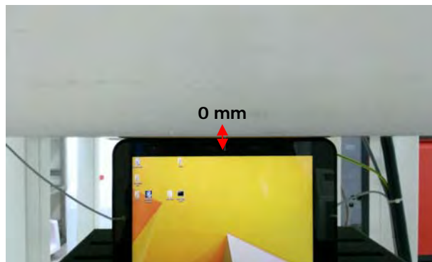
Fig.6 EUT Right side to flat phantom
