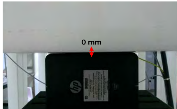
Fig.4 EUT Top side to flat phantom
