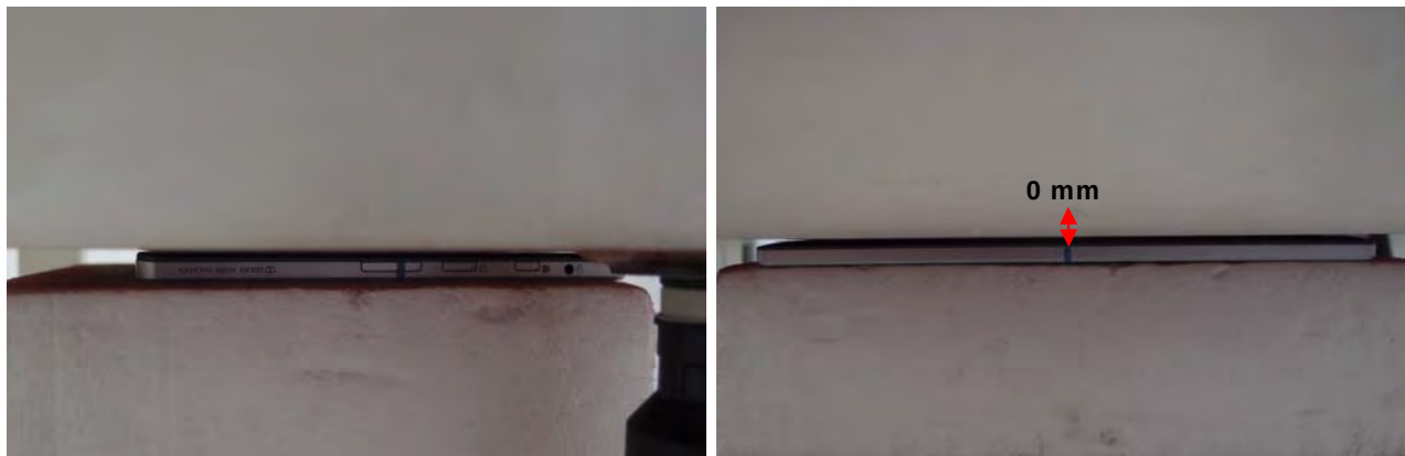
Fig.3 EUT Lap-held mode to flat phantom
