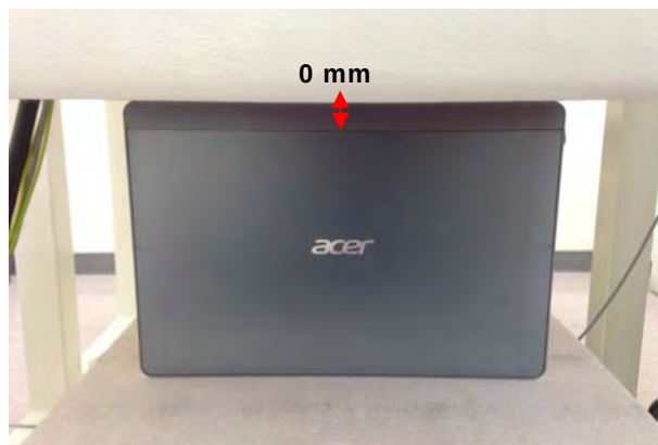
Fig.4 EUT Top side to flat phantom
