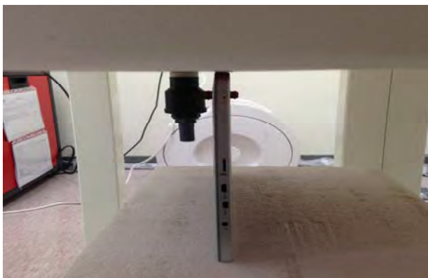
Fig.4 EUT Top side to flat phantom
