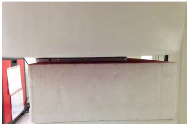
Fig.3 EUT Lap-held mode to flat phantom
