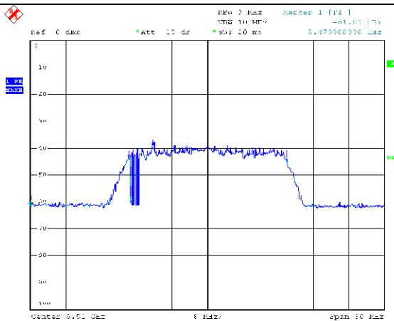
**EUT (Client ) links with master on 5510MHz**
