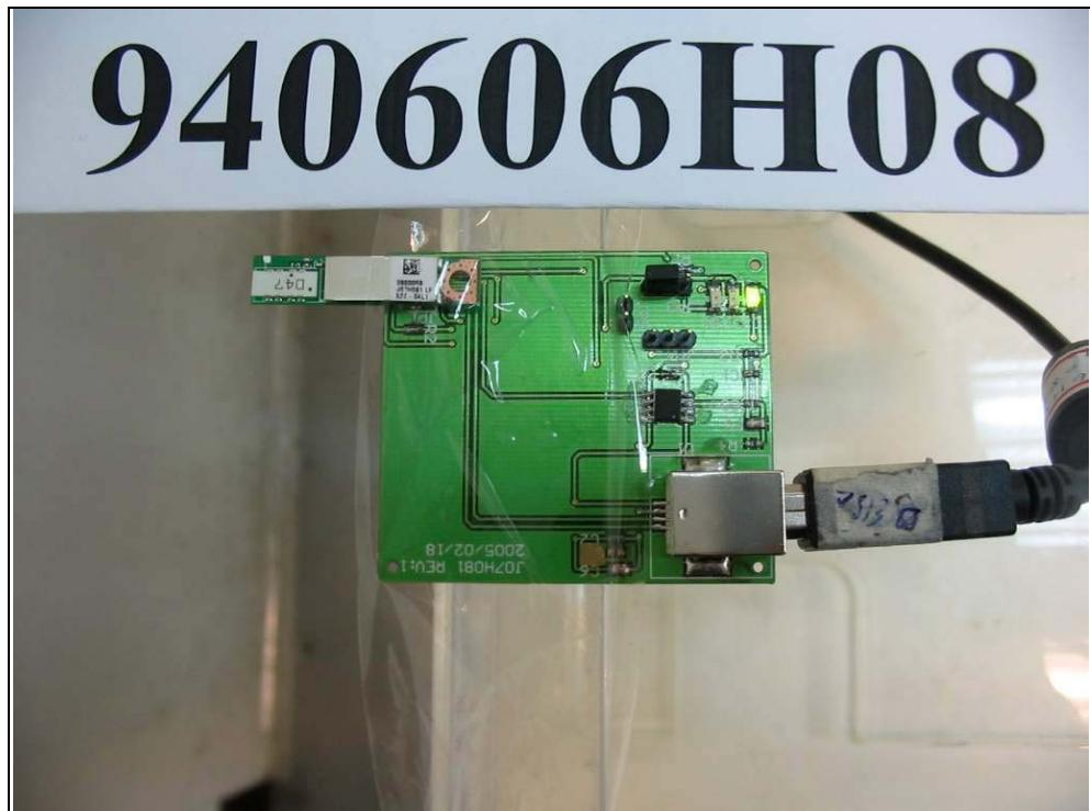
RADIATED EMISSION TEST (X axis)
