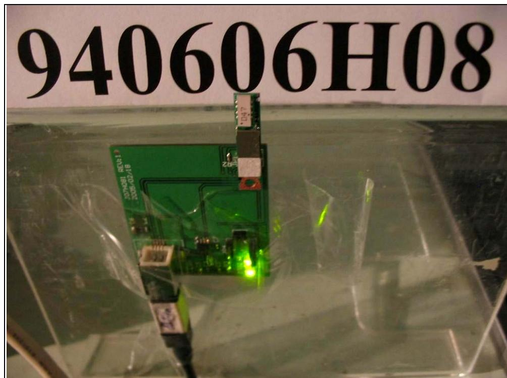
RADIATED EMISSION TEST (Z axis)
