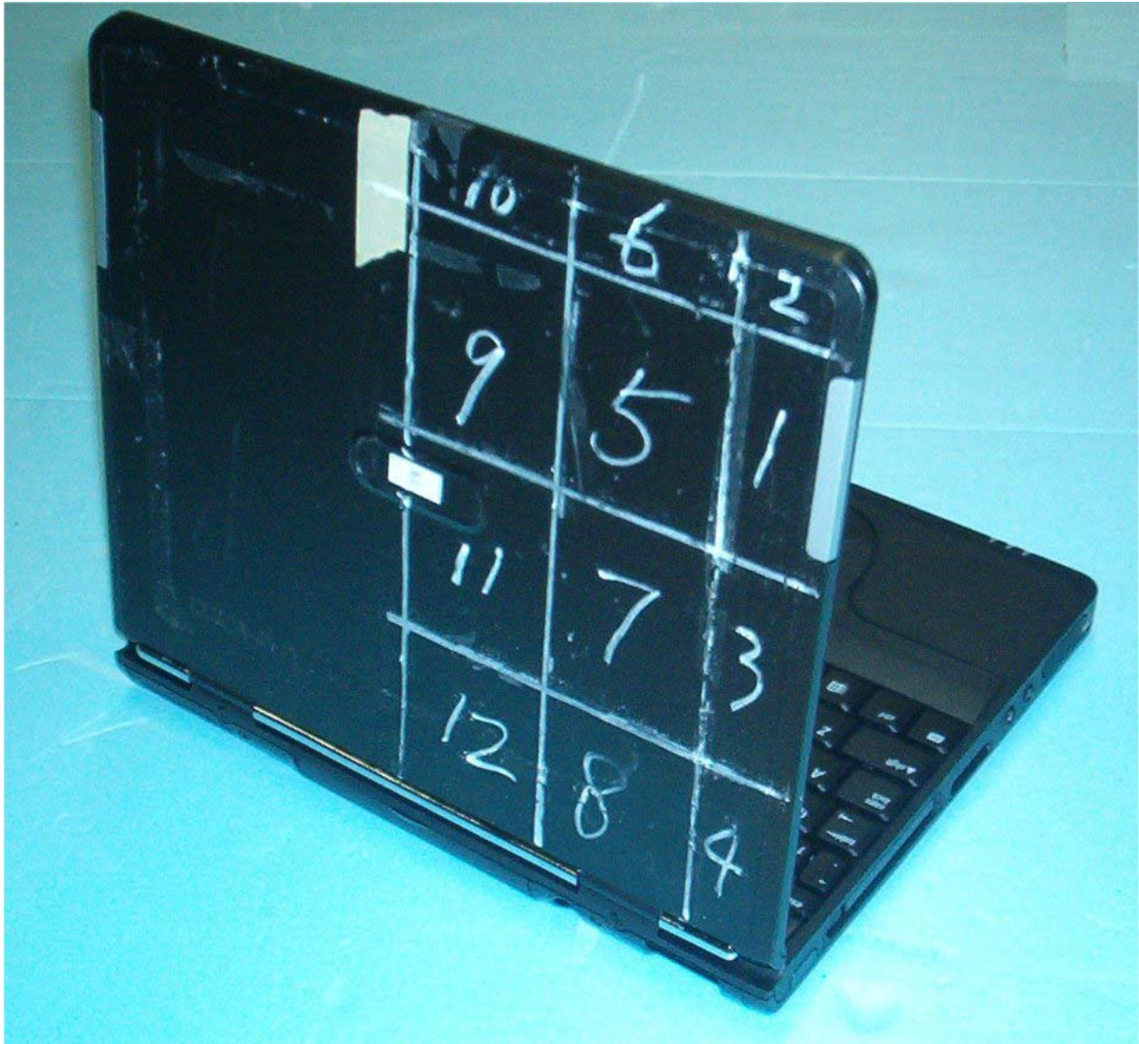
Fig. f. Photograph of the top cover to the Agency Series Laptop Computer with built-in Ambit Microsystems 802.11 a/b Wireless Antennas A and B. Marked here as the various regions 1-12 close to and including the higher SAR Antenna B, each of dimension 5.6 \times 8.0 cm that have been scanned for SAR distributions with a coarse scan resolution of 0.8 cm (8 mm).
