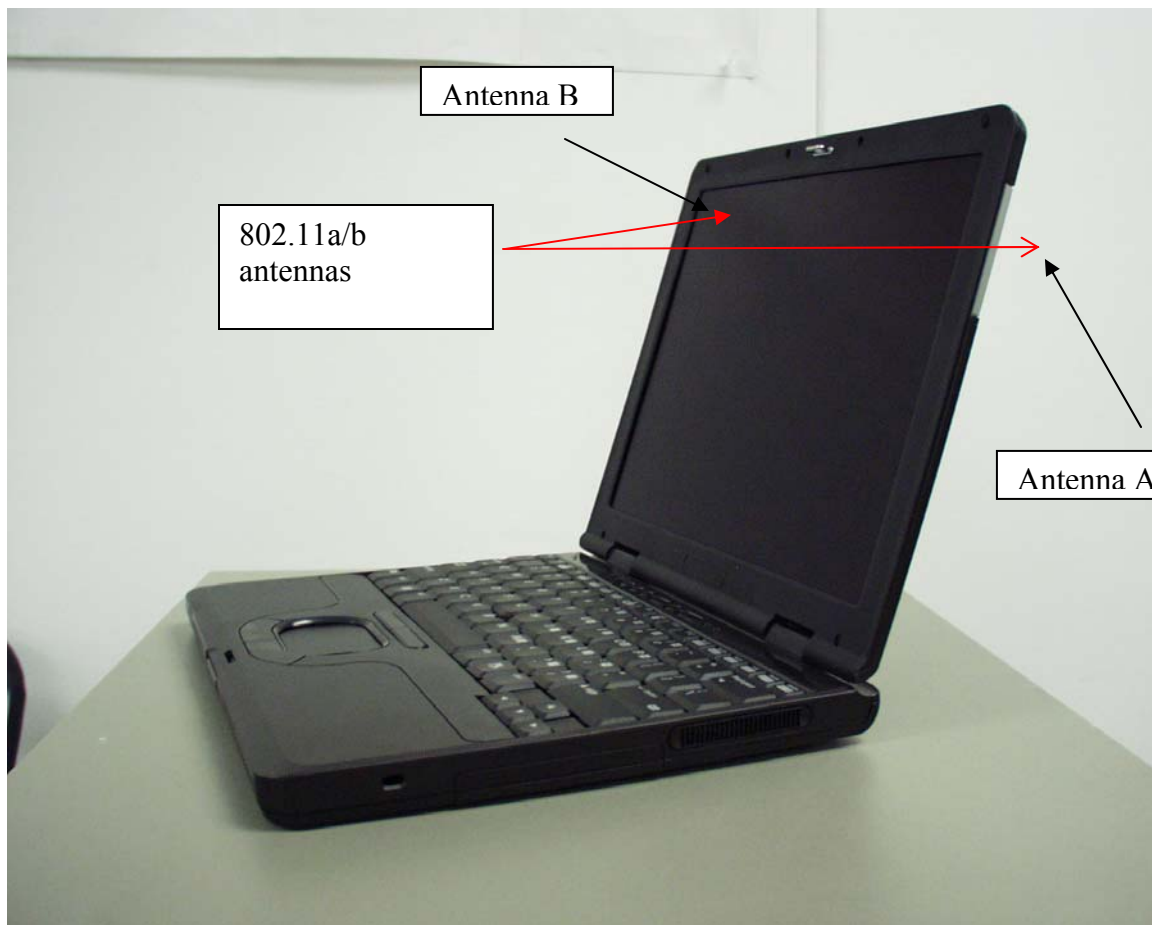
Fig. a. A photograph of the Agency Laptop Computer showing the placement of the Ambit Microsystems 802.11 a/b Wireless Antennas against the two sides of the lid with the computer screen. (This is a corrected version of the previously submitted Fig. 2 where a Bluetooth Antenna, not used for this PC, was shown by mistake).
