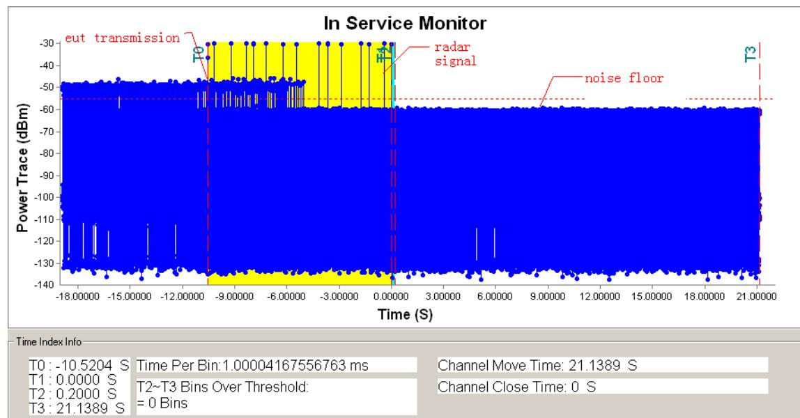
**Note:** T1 denotes the start of Channel Move Time upon the end of the last Radar burst.
