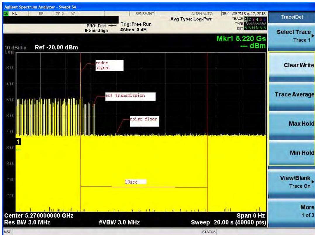
**Note:** An expanded plot for the device vacates the channel in the required 500ms
