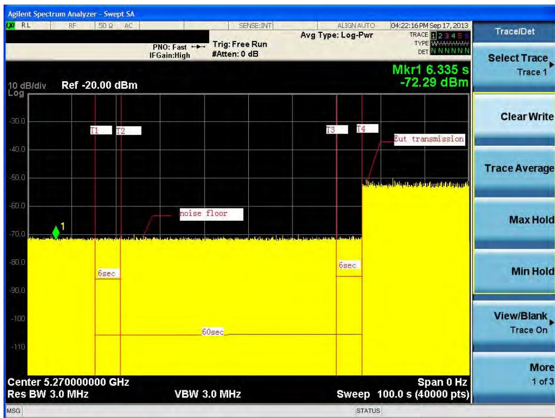
**Note:** T1 denotes the end of power-up time period is 14 second. T4 denotes the end of Channel Availability Check time is 74 second. Channel Availability Check time is equal to (T4 – T1) 60 seconds.
