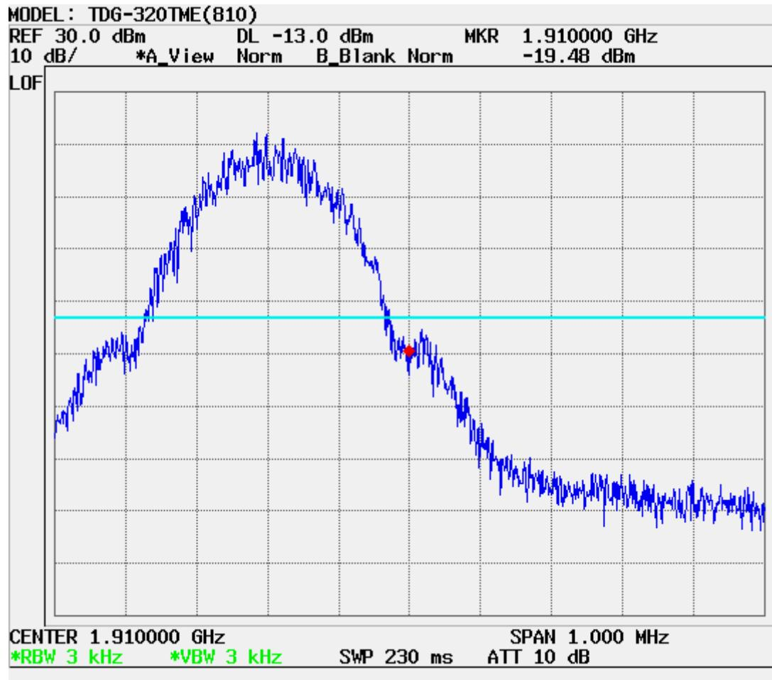
**■ Power output conducted (GSM1900 512 CH)**
