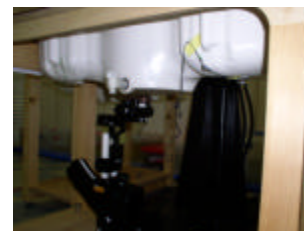
Fig. 18. Body SAR Test Setup with Holster
