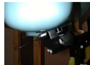
Figure 18. Right Head SAR Test Setup -- Check / Touch Position --
