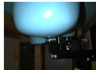
Figure 19. Right Head SAR Test Setup -- Ear / Tilt Position --
