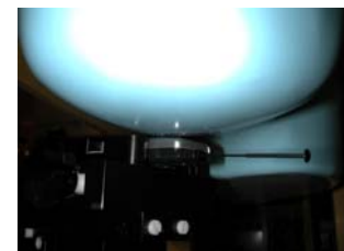
Figure 17. Left Head SAR Test Setup -- Ear / Tilt Position --
