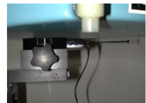
Figure 20. Body SAR Test Setup
