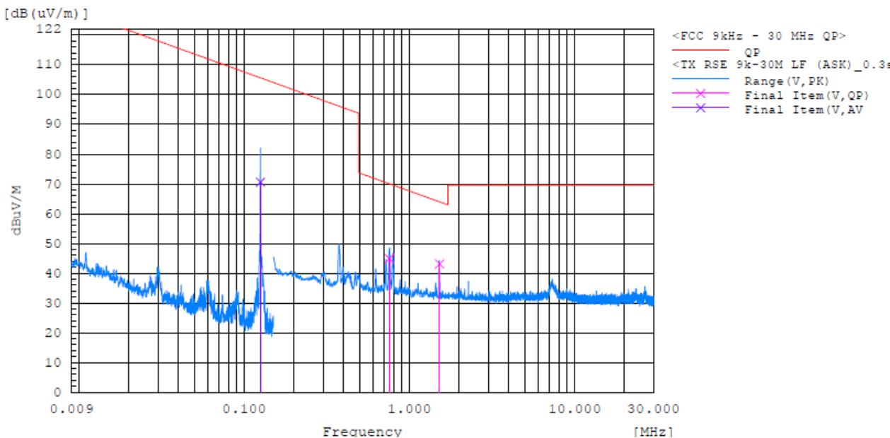
**Radiated Spurious Emission 9 kHz – 30 MHz (Antenna Position 180°) : LF (ASK)**
