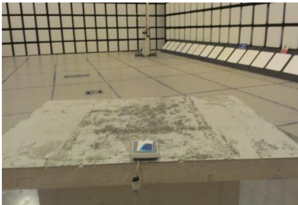
Figure 9: RE test setup for 30MHz to 1GHz – Vertical – Identive Cloud 4710 F
