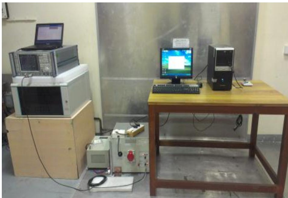
Figure 10: Conducted Emissions test setup
