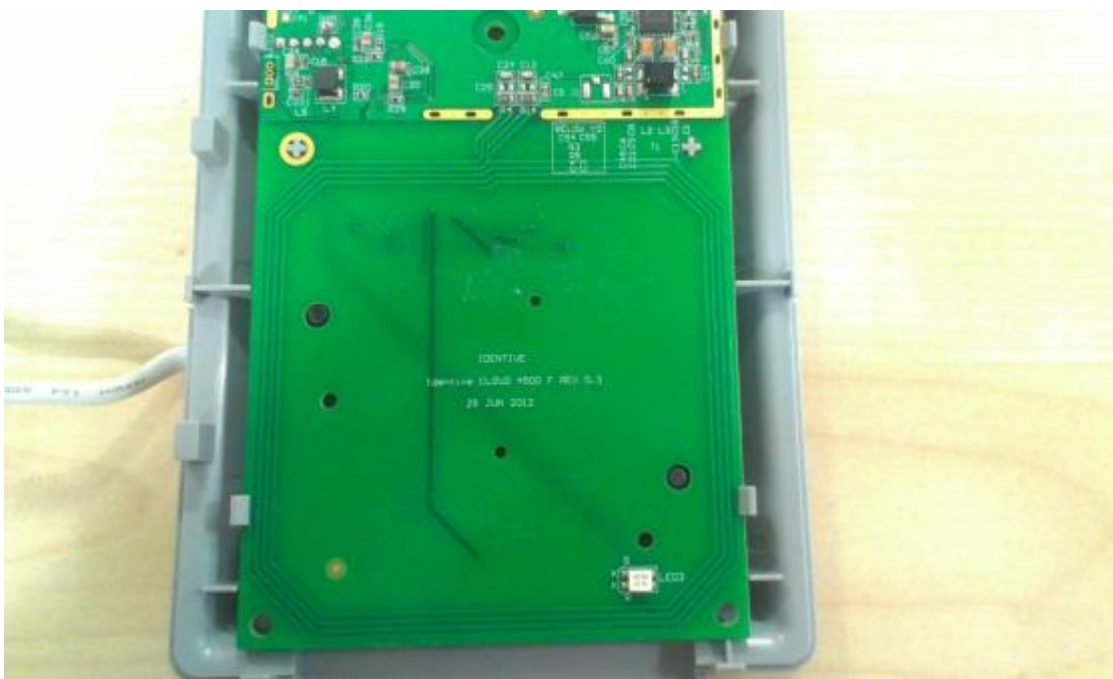
Figure 3: Photograph showing onboard antenna for Intentional Radiation
