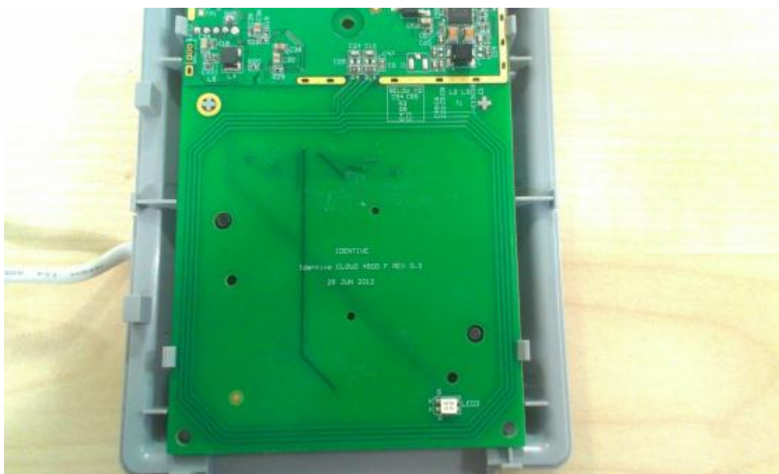
Figure 4: Photograph showing onboard antenna for Intentional Radiation
