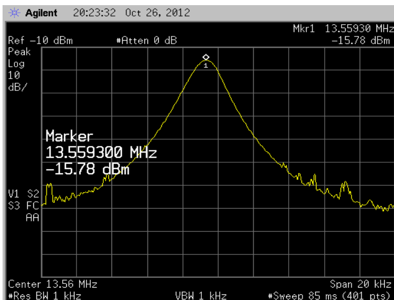
Figure 35: Carrier Frequency at 20°C for 5VDC input voltage
