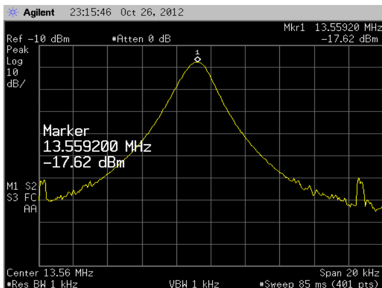
Figure 41: Carrier Frequency at 20°C for 5VDC input voltage
