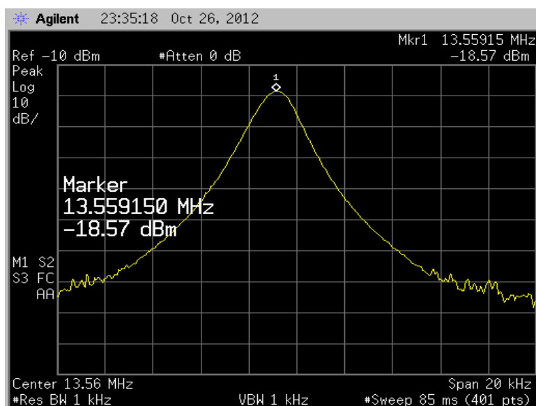
Figure 42: Carrier Frequency at 50°C for 5VDC input voltage
