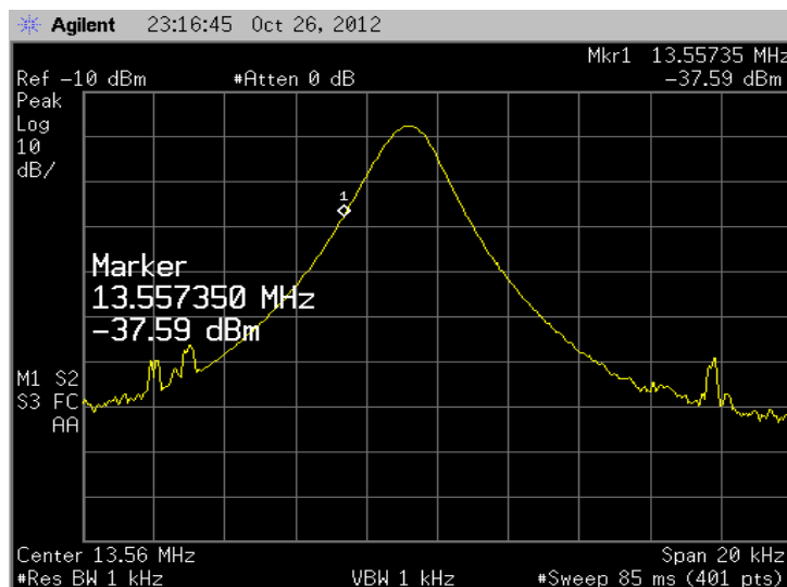
Figure 28: Measured f_L for 20dB Bandwidth
