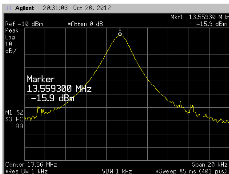
Figure 40: Carrier Frequency at 20°C for 5.75VDC input voltage
