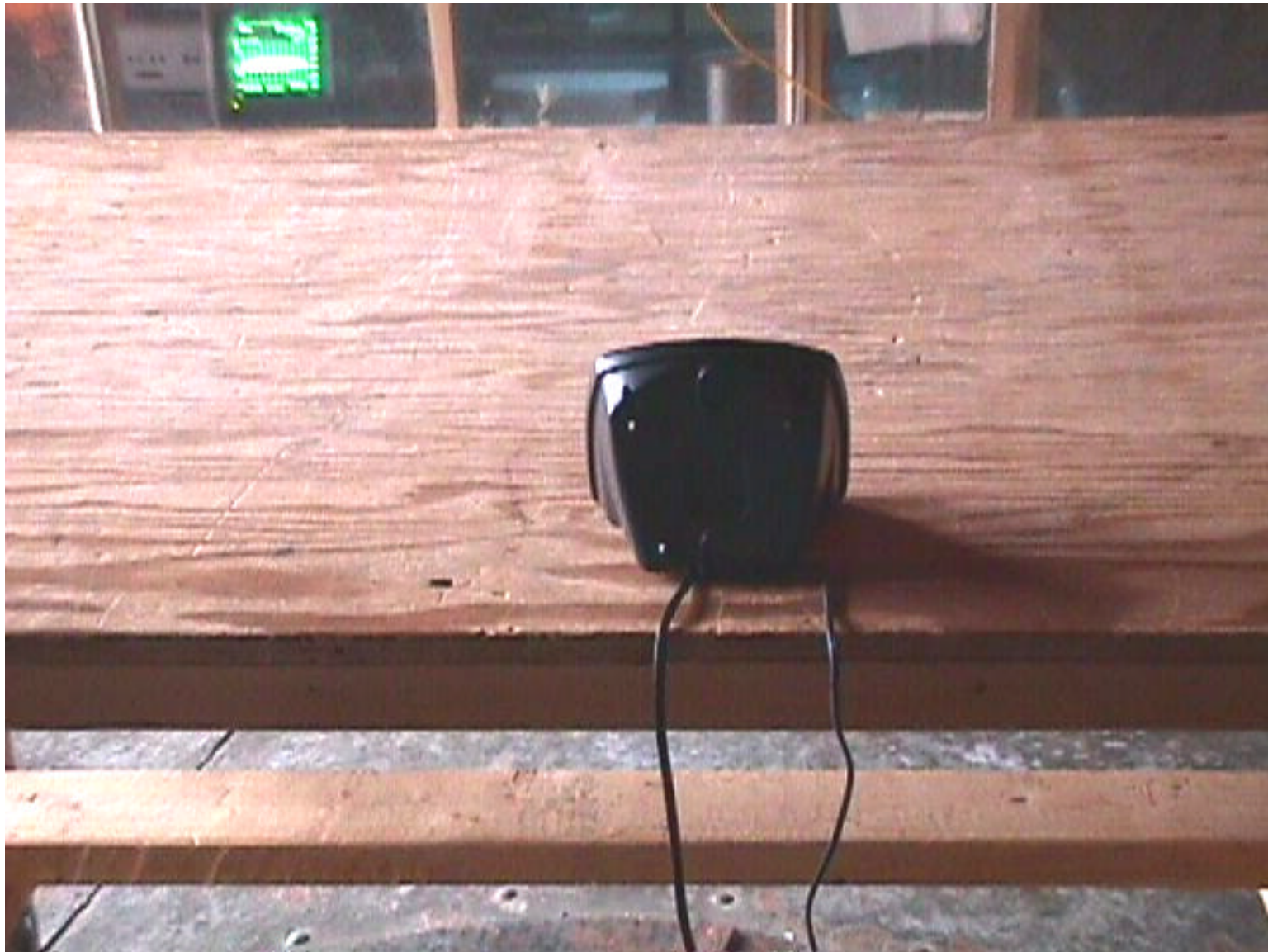
Test Setup for Radiated Emissions - Base Unit
