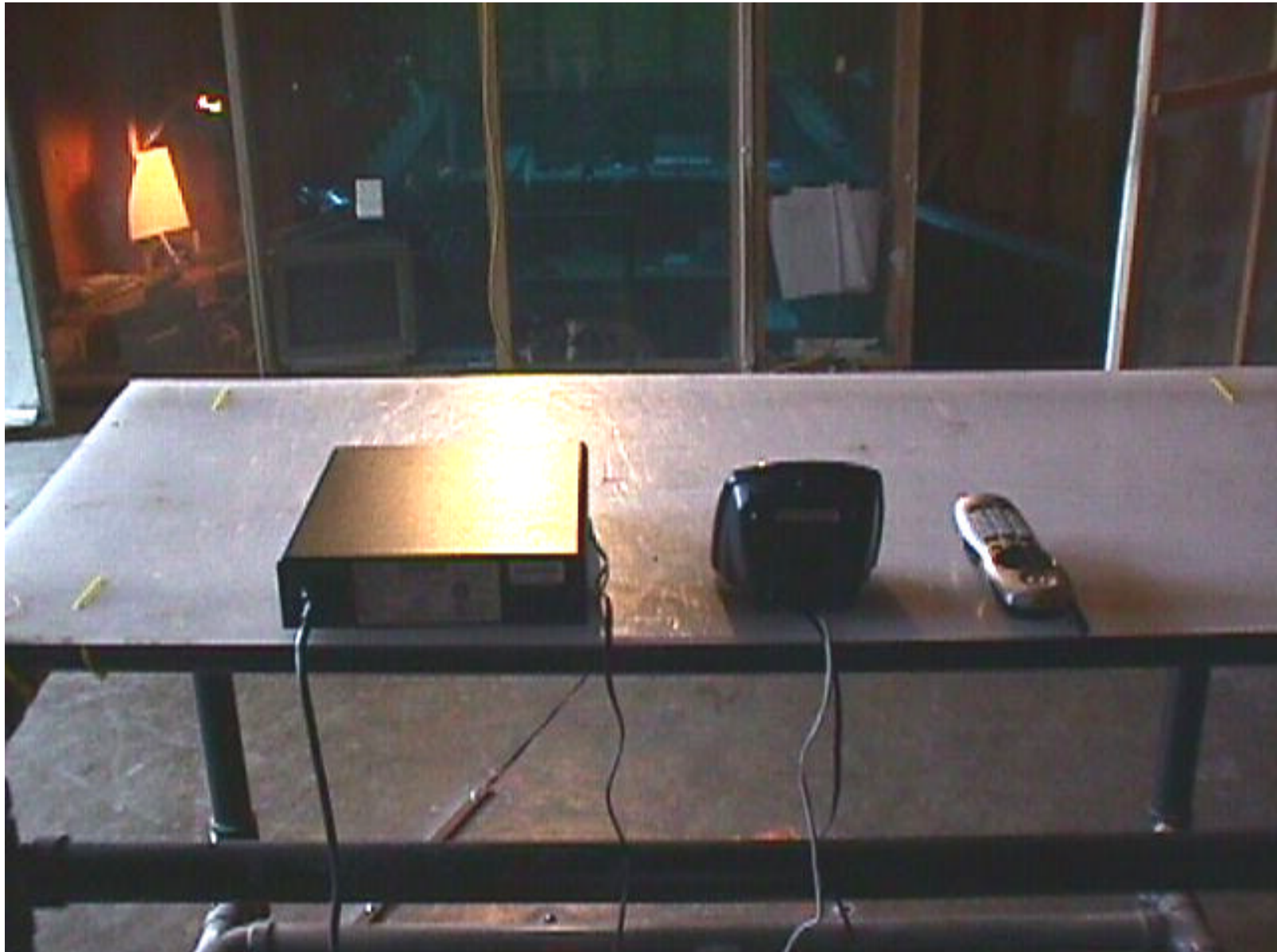
Test Setup for Digital Apparatus Radiated Emissions - Handset & Base Units
