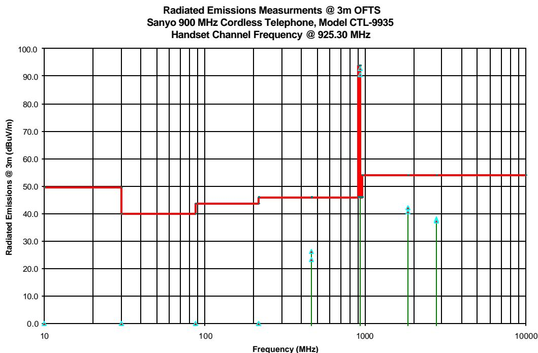
**6.8.1.4. Transmitter Radiated Emissions from Handset Transmitter @ Highest Channel Frequency: 927.25 MHz**
