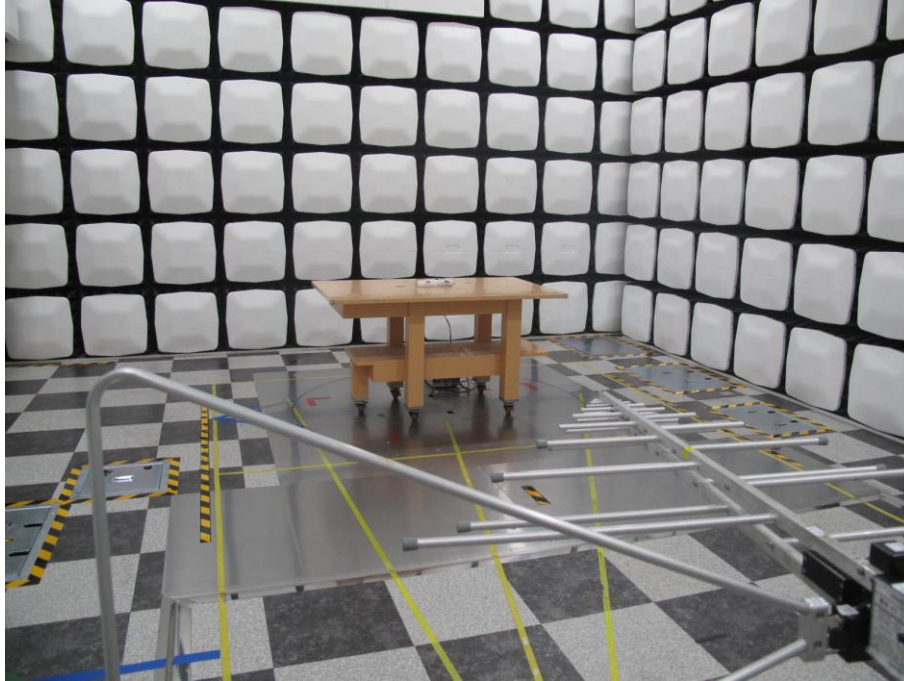
Radiated Test Picture(Front)_ Dipole Ant_Below 1GHz
