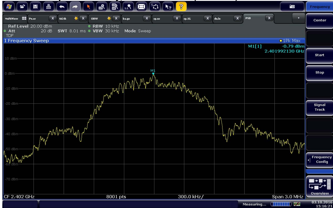
Peak Power Spectral Density, Lowest Channel (2402 MHz)
