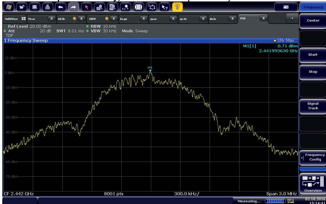
Peak Power Spectral Density, Middle Channel (2442 MHz)
