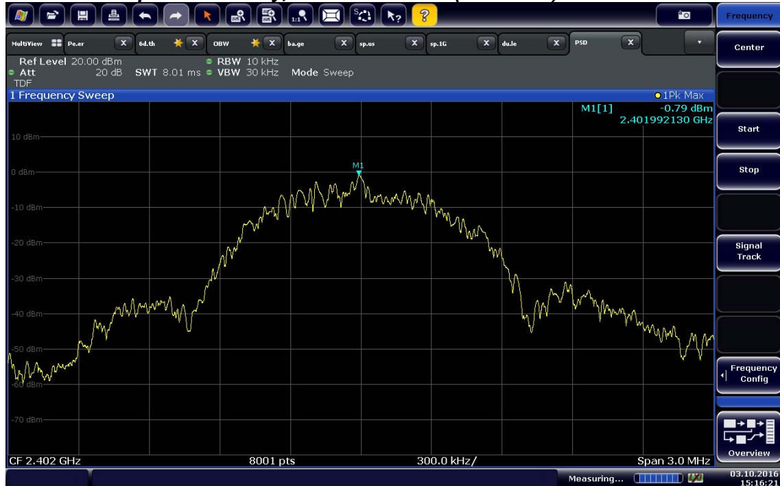
Peak Power Spectral Density, Lowest Channel (2402 MHz)
