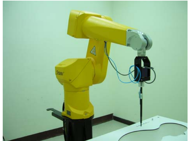
Fig. 5.2 Probe Setup on Robot
