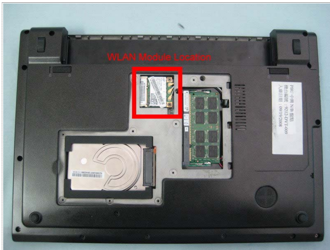
WLAN module Location
