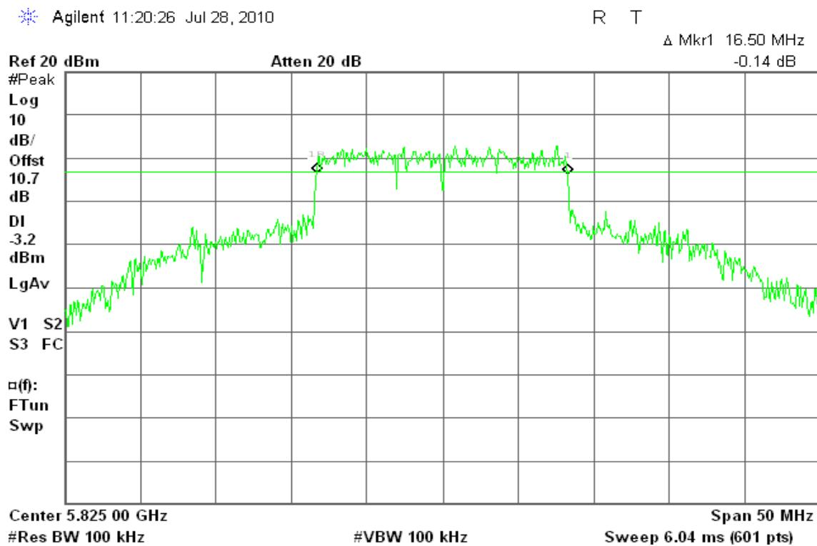
**draft 802.11n Standard-20 MHz Channel mode****6dB Bandwidth (CH Low)**
