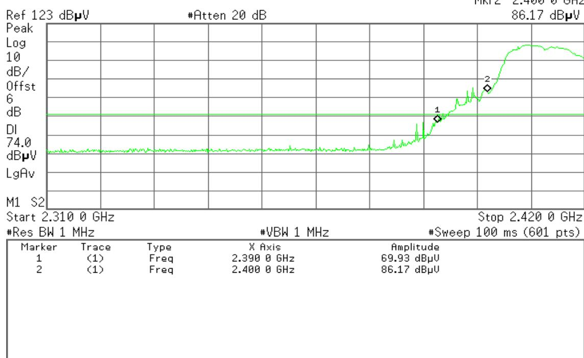
**Detector mode: Average****Polarity: Horizontal****\* Agilent 17:14:55 Sep 27, 2010**
