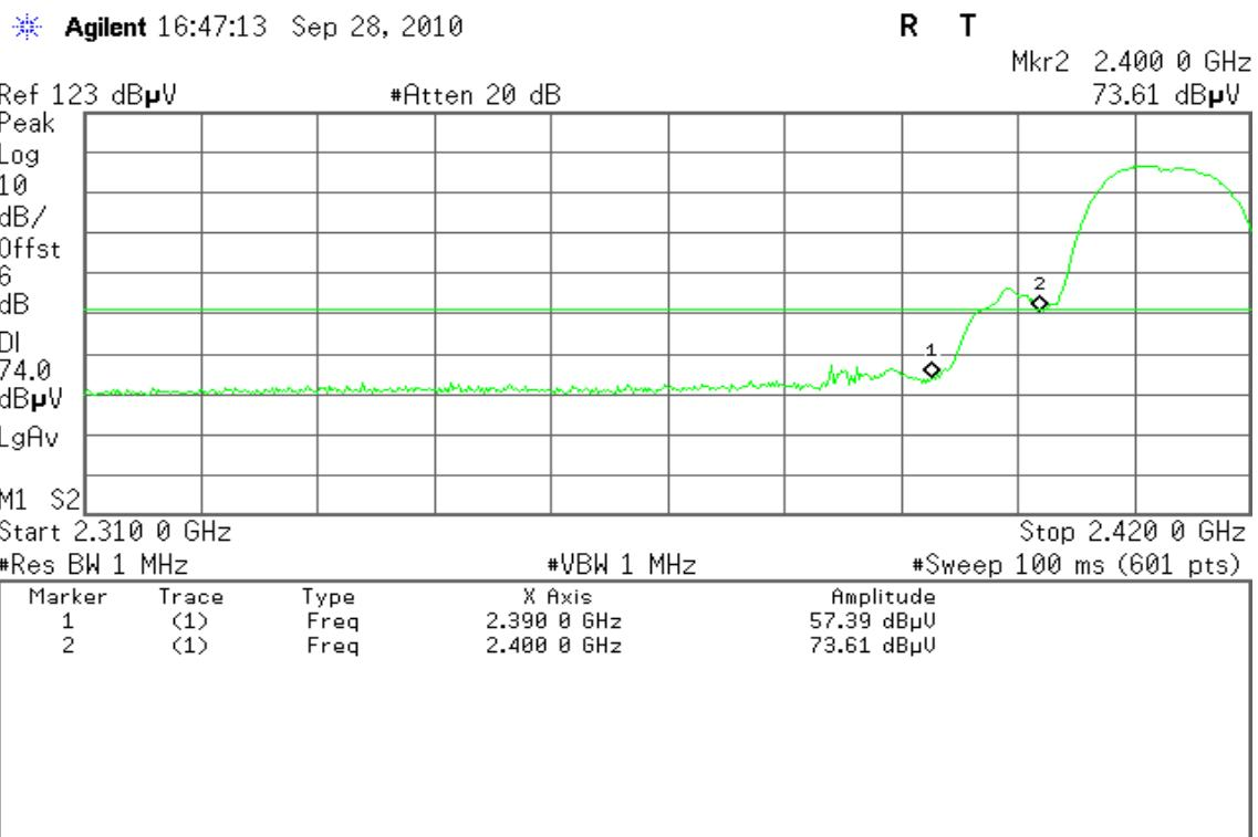
**Detector mode: Average****Polarity: Horizontal**
