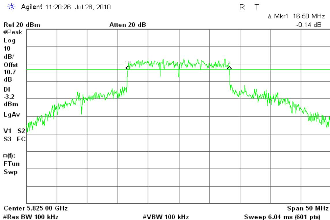
**draft 802.11n Standard-20 MHz Channel mode****6dB Bandwidth (CH Low)**
