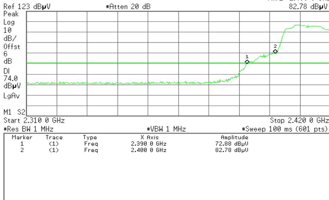
**Detector mode: Average****Polarity: Horizontal****\* Agilent 10:11:36 Sep 28, 2010**
