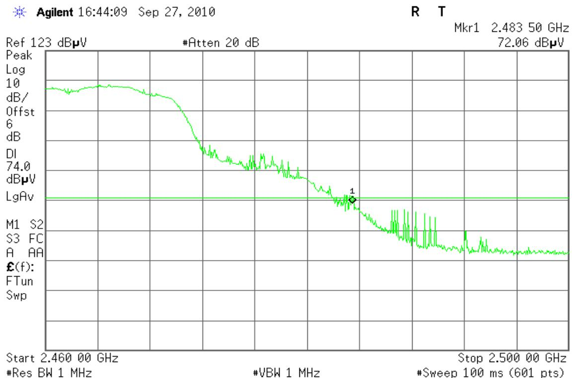
**Detector mode: Average****Polarity: Horizontal**
