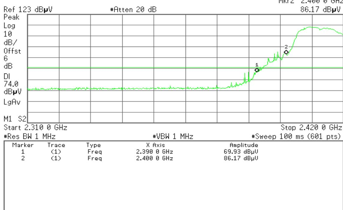
**Detector mode: Average****Polarity: Horizontal****\* Agilent 17:14:55 Sep 27, 2010**
