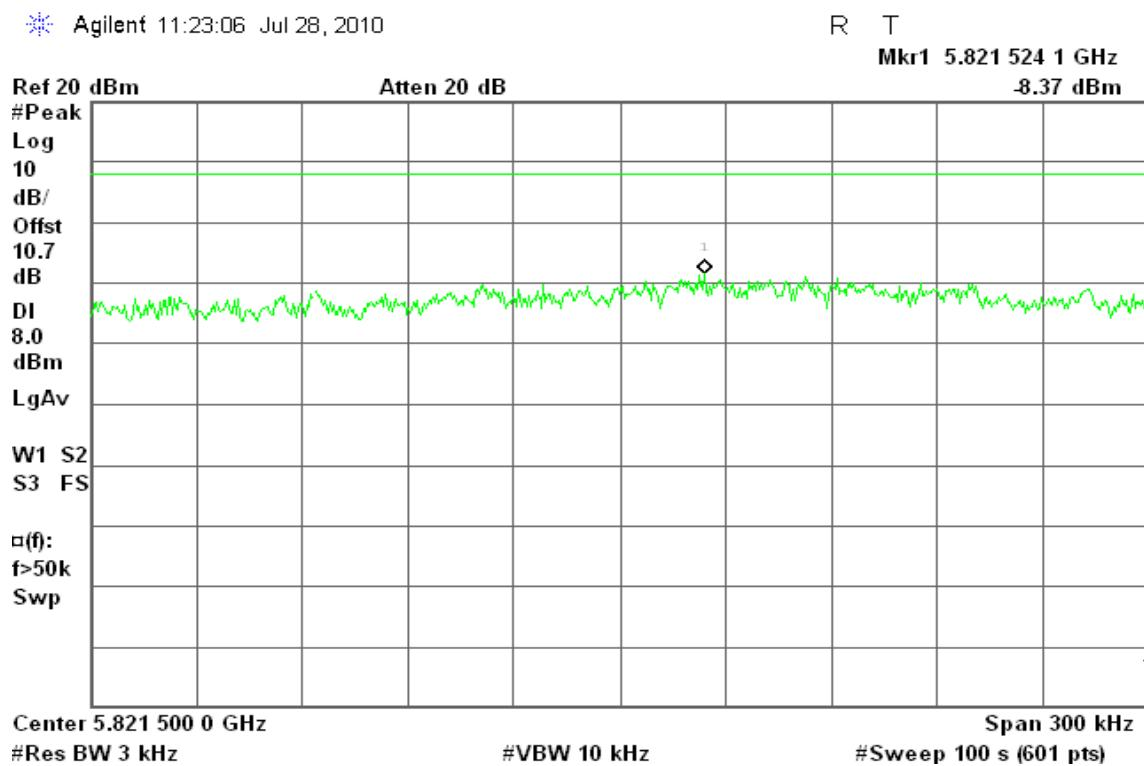
**draft 802.11n Standard-20 MHz Channel mode****PPSD (CH Low)**
