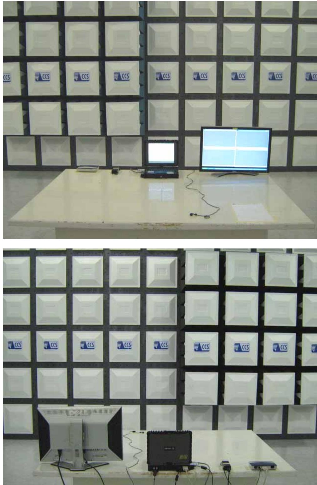
**POWERLINE CONDUCTED EMISSIONS MEASUREMENT SETUP****EMC-1**
